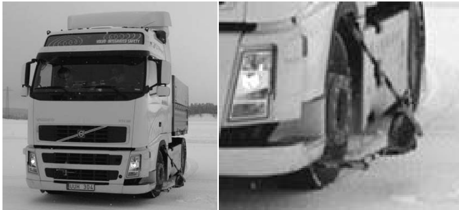
Figure 8 Test vehicle Volvo FH12 with tyre sensor receiver unit next to left front wheel
