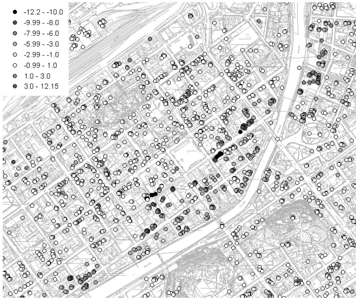
Figure 3 Coherent targets in Turku with some base map data. The vertical motion rates are in millimetres per year.
