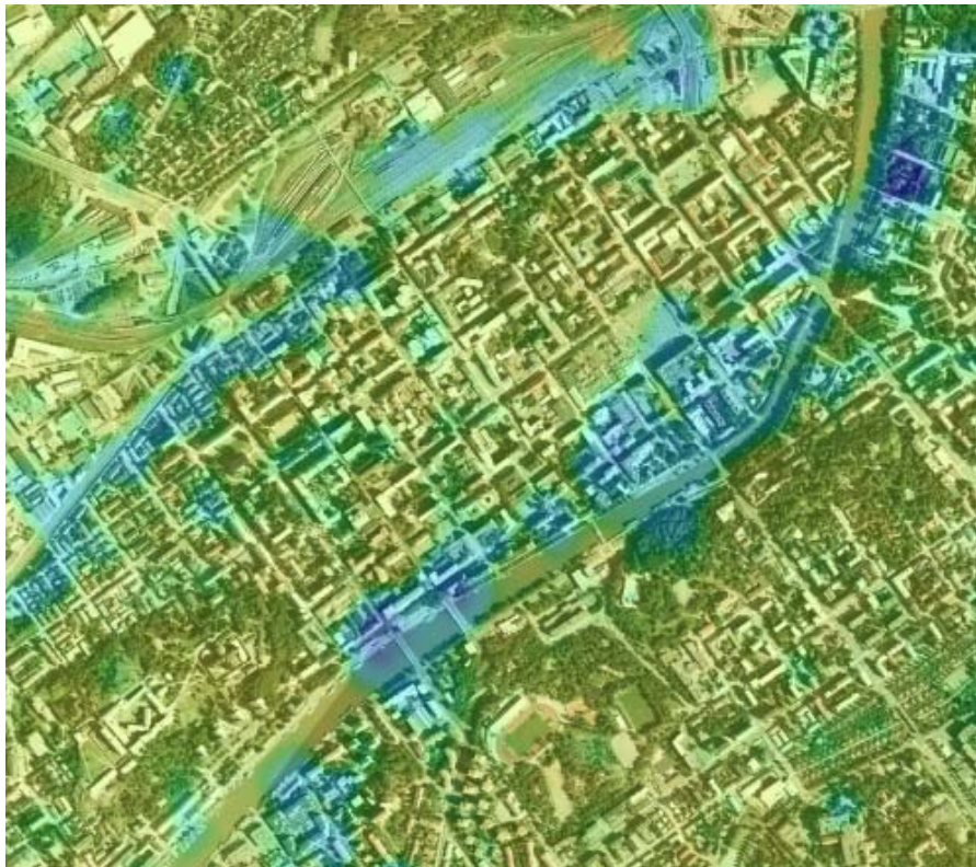
Figure 6 An interpolated subsidence map of Turku. The blue areas subside.
