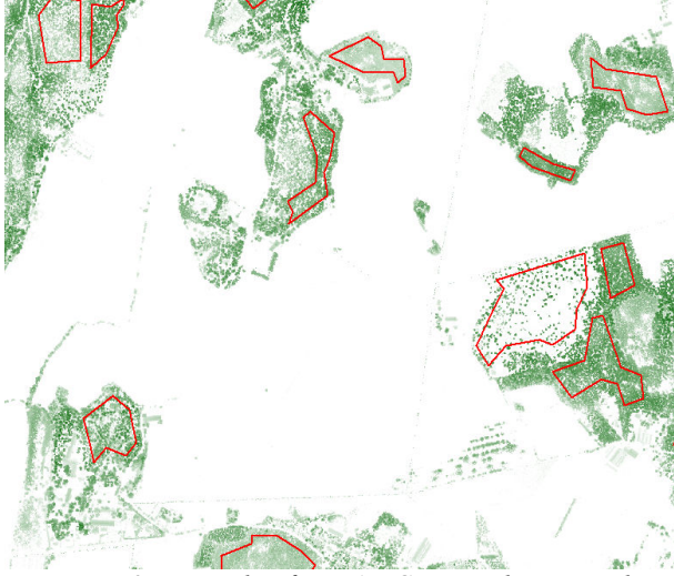
Figure 2. Example of LIDAR CHM and test stands (White corresponds to ground level and dark green is approximately 35m above ground).
