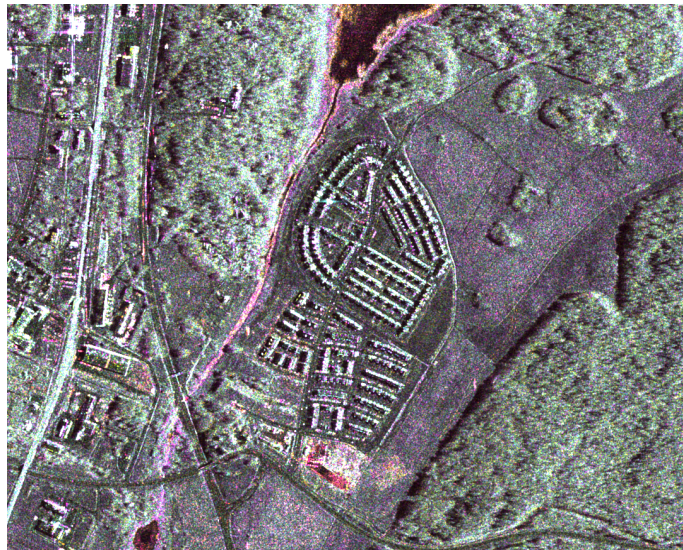
Figure 2. Masala, Finland, seen by TerraSAR-X satellite (Image data 2008-2009 © DLR, multitemporal images, nominal resolution: 2.0 m (ground range) and 2.3 m (azimuth), High Resolution Spotlight Mode, Dual polarization).
