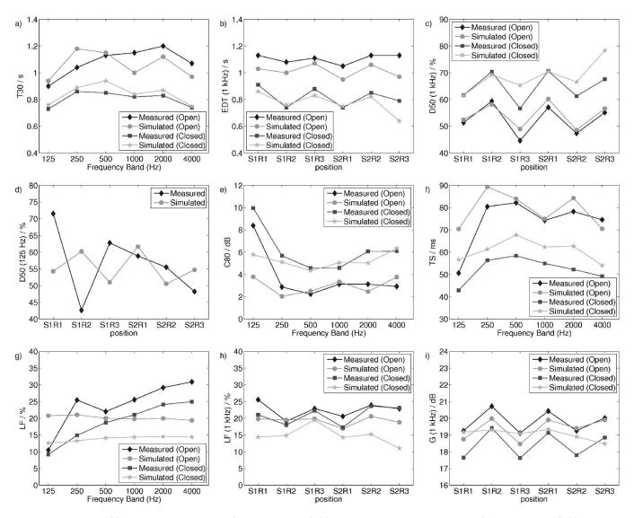
FIG. 6. The charts show (a)  $T_{30}$  values at position S2R2 (cf. Fig. 6 in Ref. 30), (b) EDT values in the 1 kHz octave band (cf. Fig. 8 in Ref. 30), (c)  $D_{50}$  values in the 1 kHz and (d) 125 Hz octave bands (cf. Figs. 10 and 11 in Ref. 30 respectively), (e)  $C_{80}$ , (f) TS, and (g) LF values at position S1R1 (cf. Figs. 13, 14, and 19 in Ref. 30, respectively), and (h) LF and (i) G in the 1 kHz octave band (cf. Figs. 20 and 17 in Ref. 30, respectively).
