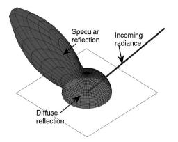
FIG. 1. A BRDF represents the directional distribution of the reflected energy for each incoming angle. Here the distribution for one angle is shown.
