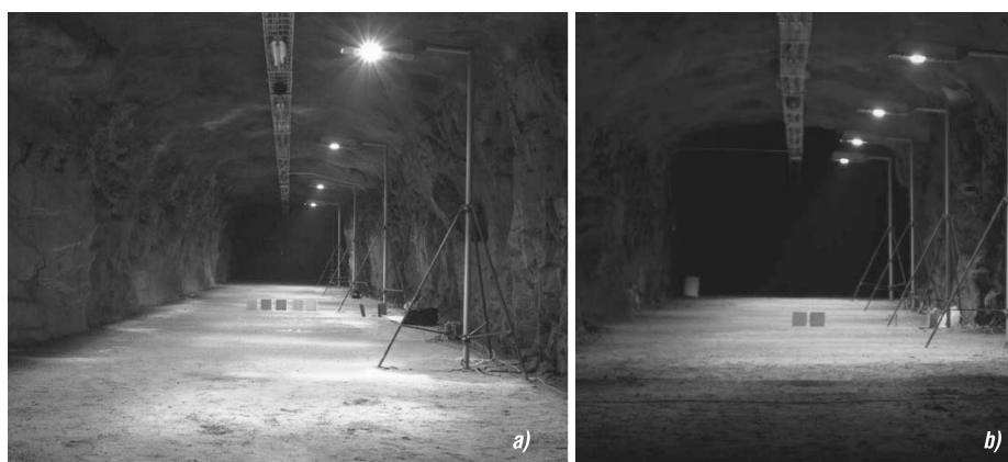
Fig. 5. Experimental set-up in the underground tunnel and two road lighting installations used in the experiments. a) Two achromatic and three coloured targets illuminated with MH lamps. b) An achromatic and a green target illuminated with HPS lamps
