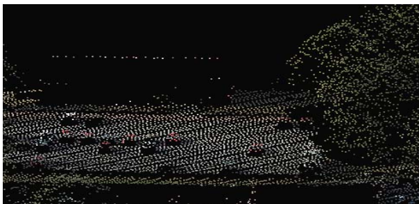
Figure 7. Top: coloured 3D ALS point cloud looks photorealistic when viewed from a distance that meets the resolution of ALS data. Bottom: the structure of the ALS point cloud becomes visible when the viewing location is close enough. The images are created with TerraScan.
