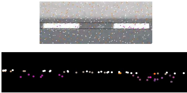
Figure 2. The cross-section of ALS data reveals how some echoes are shifted downwards from the asphalt level when hitting the white road markings.
