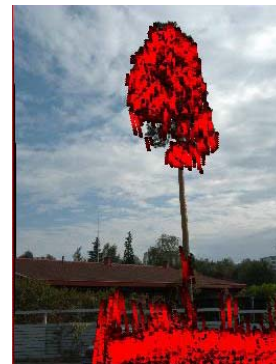
Figure 15. Full-waveform ALS data is superimposed onto the terrestrial image (Litkey et al., 2007).
