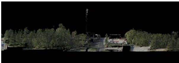
Figure 9. Typical integration of orthoimage and an ALS point cloud (TopoSys-1).
