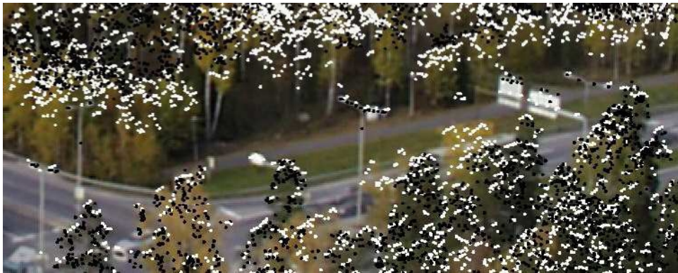
Figure 8. White spots are scanned from 800 m with the pulse repetition rate of 83 kHz (airborne TopoSys-1) and black points are scanned from 200 m at the rate of 7 kHz scanning rate (helicopter-borne TopEye).
