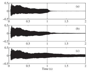
Fig. 1. Sound waveforms of the piano tone G3 ( $f_0$ =196.4 Hz) played (a) without the sustain pedal, (b) with part-pedaling, and (c) with full sustain pedal. The curves are aligned at key release (vertical lines), defined as the time instant when the key reached the upper position.
