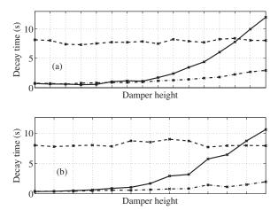
Fig. 3. Decay rates of the three time intervals of the decay (see text) as a function of the damper height adjustment for two piano tones (a) G2 ( $f_0$ =98.12 Hz) and (b) G3 ( $f_0$ =196.4 Hz): initial free vibration (dashed line), damperstring interaction (dash-dotted line), and final free vibration (solid line). Each adjustment step (grid line) corresponds to 0.08 mm.
