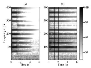
Fig. 4. Spectrograms of the tone C1 ( $f_0$ =32.54 Hz) played (a) with part-pedaling and (b) with full pedal. The vertical lines show the duration of the damper-string interaction when part-pedaling is used. The same interval is shown in (b) for reference.
