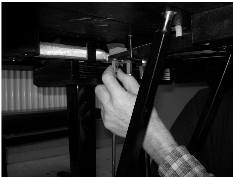
Figure 6.4: Prof. Askenfelt turning the sustain pedal rod nut that controls the distance between the strings and the dampers.
