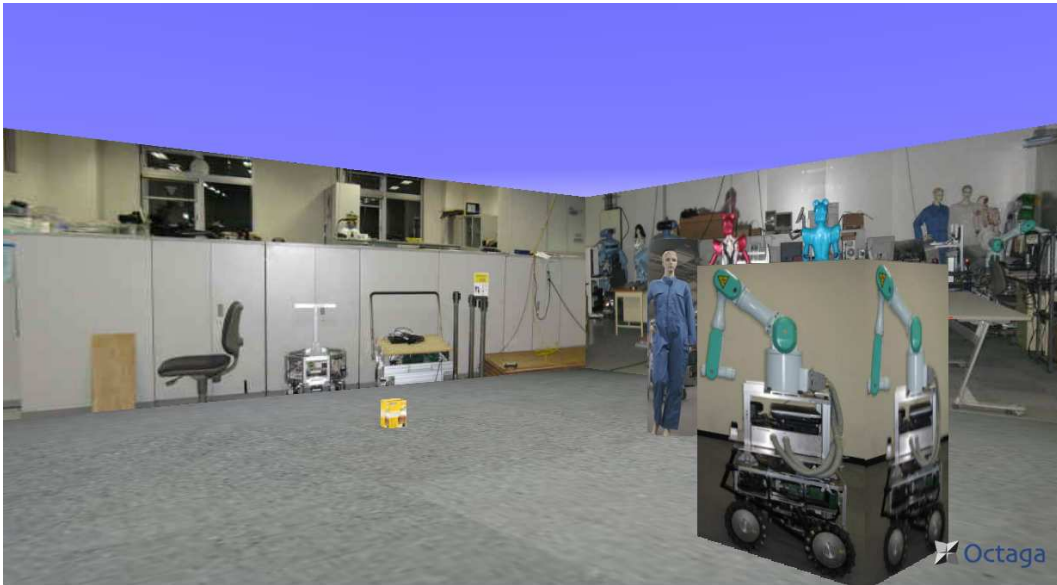
Figure 5.4: View of X3D file created from database as a snapshot of the robot's understanding of the world
