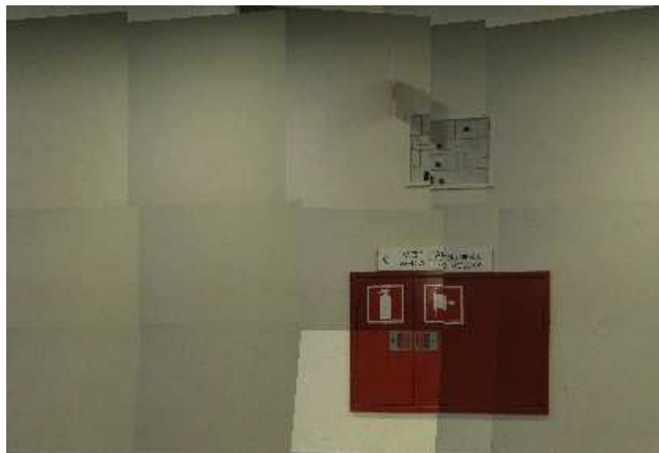
Figure 7.17: A sample of a stitched wall segment texture: The stitch marks in the image are due to the auto gain of the camera but it can still be used as a texture map.
