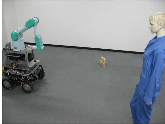
Figure 7.5: Experimental setup for MARY in pose reservation experiment
