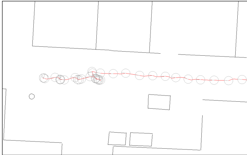
Figure 7.16: Path of Rolloottori robot while texturing a wall segment: the robot approaches from the right and stops at five locations to take images
