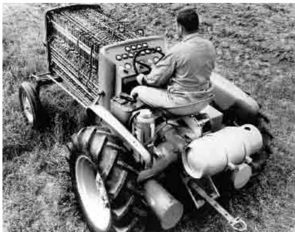
Figure 1. An experimental Allis-Chalmers fuel cell tractor in 1959 [7].
