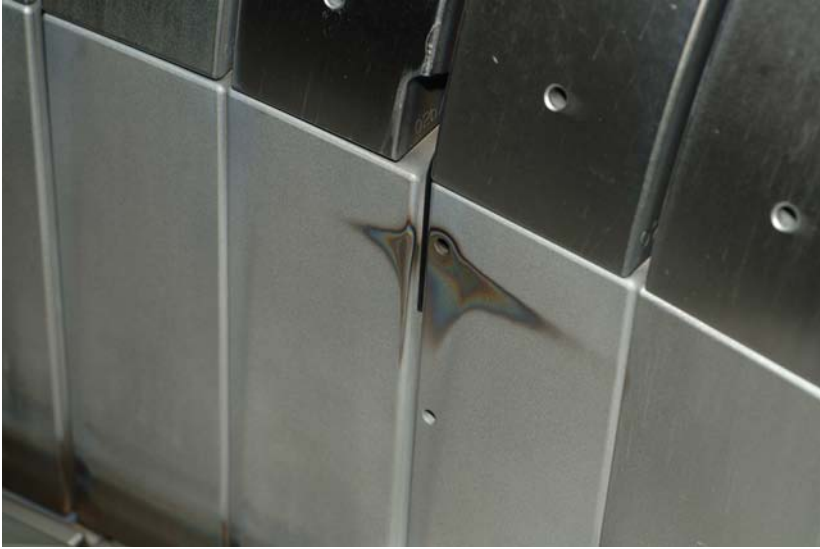
Figure 3.2: ^{13}\text{C} deposition pattern in the divertor in the 2008 experiment with a reduced injection rate. Figure courtesy of V. Rohde / IPP Garching.
