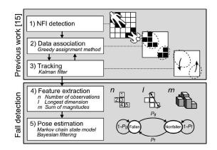
Fig. 1. Process flow of the NFI fall detector.
