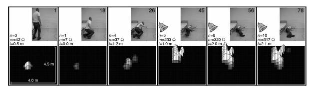
Fig. 2. Example of fall detection with the NFI floor sensor. Video (30 fps) and NFI data were recorded simultaneously. The bell indicates the fall-alarm state.
