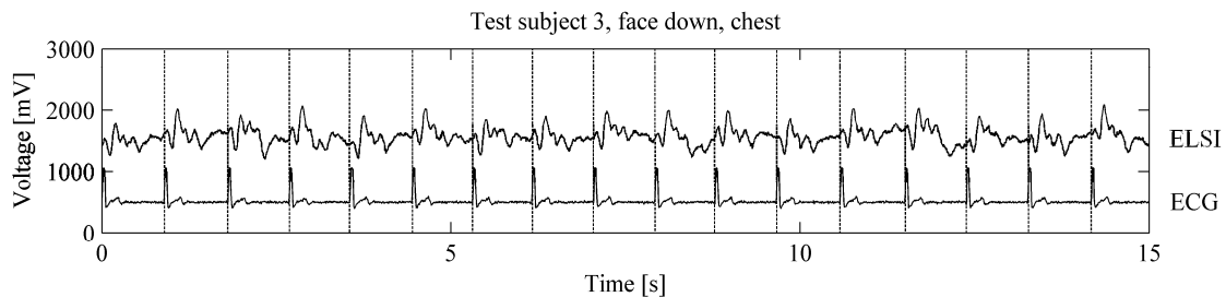
Figure 24. Cardiac signal of one test subject. He was lying prone and the signal was recorded at chest height.
