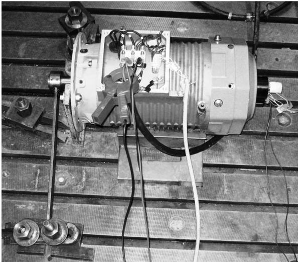
Fig. 7. The test setup. The rotor was locked by the bar on the left during the demagnetization test.
