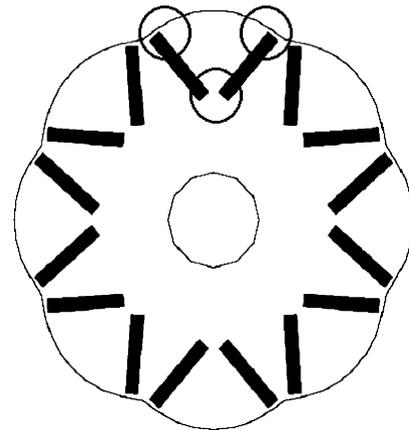
Fig. 1. A conventional buried magnet machine. The iron pole between the magnets is supported by thin iron bridges, which are kept thin because of the leakage flux. The centrifugal forces acting on poles in higher speeds are causing stress on the iron bridges (circled in one pole).
