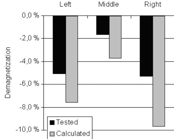
Fig. 8. A measured demagnetization (drop of magnetic polarization) of the poles after the locked-rotor situation with a 100 Hz, 165 A input compared to the calculated demagnetization. This machine had a single-grade construction with grade A only. The mass of the middle magnet is twice the mass of the side magnet.
