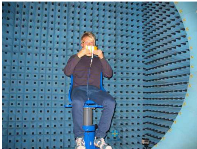
Fig. 7. Efficiency measurement for the browsing grip with the Satimo Stargate measurement system.
