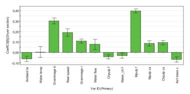
Figure 7. Scaled predictor coefficients in 2004 and 2007 PLS models for the paper machine dryer section during normal operation
