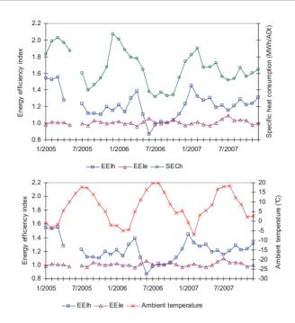
Figure 5. Monthly energy efficiency indices of the case paper machine
