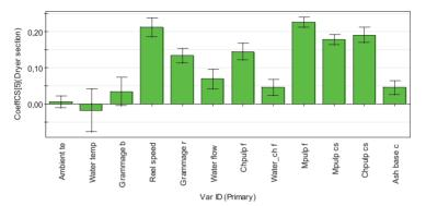
PLS analysis of dryer section 2004.M9 (PLS), PLS2004operation CoeffCS[Comp. 5](YVar Dryer section)
