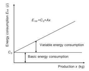
Figure 1. Division of basic and variable energy consumption (reproduced from [3])
