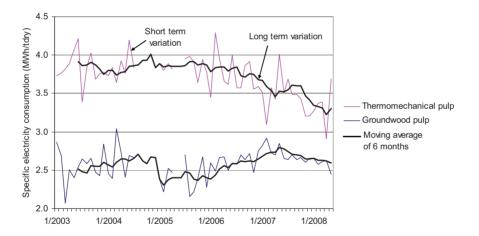
Figure 3. Moving averages of specific electricity consumption of two mechanical pulp plants
