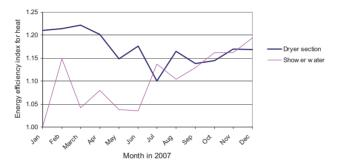
Figure 6. Operation time energy efficiency indices for heat consumption in the dryer section and shower water heating in 2007 using the 2004 PLS model as the baseline
