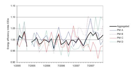
Figure 8. Aggregated energy efficiency index of electricity consumption for paper machines
