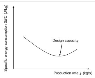
Figure 2. Specific energy consumption as a function of the production rate
