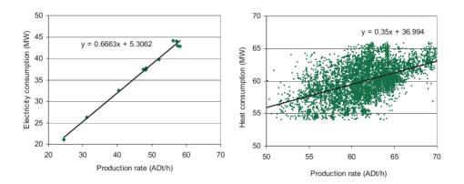
Figure 4. Correlations between energy consumption and the production rate in the case paper machine
