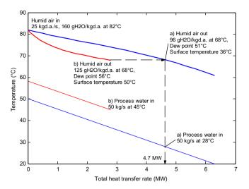
**Fig. 3.** The humidity of air after each match (here case a or b) at a certain temperature interval of the air (here 82–68 °C) is unique if condensation occurs.
