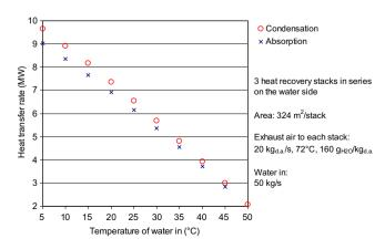
**Fig. 2.** Heat transfer rates for an example heat recovery system by using mass transfer equations for condensation and absorption: average difference 6%.
