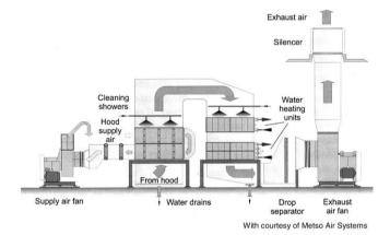
Fig. 1. Modern heat recovery stack of a paper machine dryer section.
