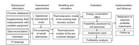
Fig. 4. Structure of the case study.
