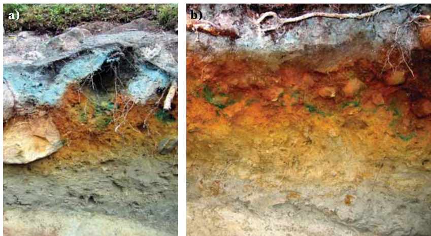
Figure 22. A vertical cross-section of dyed, unsaturated soil (a), and a cross-section of saturated soil, where the dye flows downhill above the water table (b). In (b), the dye pulse is flowing straight out of the picture.
