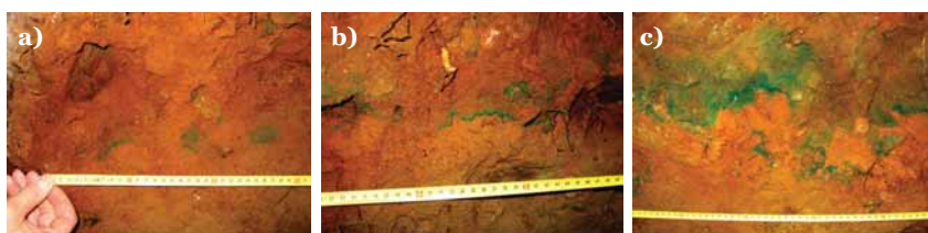
Figure 23. Continuity of the dye pulse at a distance of 120 cm (a), 60 cm (b), and 0 cm (c) from the line-type dye source in saturated soil. In the vertical cross-cut pictures, the dye pulse is flowing straight out of the picture.
