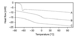
Figure 2. Glass transition points observed in DSC heating sequences for the amorphous polymers, A) PPO pre-polymer, B) PDM reference, and C) PDM-PPO-PDM
