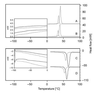
Figure 3. DSC cooling curves of A) PEO, PDM-PEO-PDM B) PEO-PPO-PEO-H, PDM-PEO-PPO-PEO-PDM-H. DSC heating curves of C) PEO, PDM-PEO-PDM D) PEO-PPO-PEO-H, PDM-PEO-PPO-PEO-PDM-H. The thicker curves are for PEO and PEO-PPO-PEO-H.
