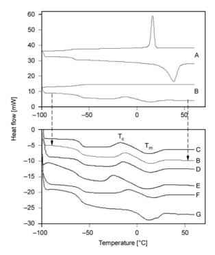
Figure 4. DSC heating and cooling curves of A) PEO-PPO-PEO-L pre-polymer, B) PDM-PEO-PPO-PEO-PDM-L. Heating curves of PDM-PEO-PPO-PEO-PDM-L with varying parameters, C) cooling -2°C/min, heating 20°C/min B) cooling -10°C/min, heating 20°C/min, D) cooling -20°C/min, heating 20°C/min, E) cooling -10°C, heating 5°C/min, and F) cooling -10°C, heating 40°C/min, G) cooling -10°C/min, heating 20°C/min after the thermal history was equalized at 40 °C.
