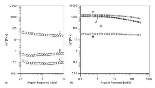
**Figure 7.** Complex viscosity of pre-polymers (a): A = PPO, B = PEO-PPO-PEO-L, C = PEO-PPO-PEO-H and modified block co-polymers (b): A = PDM-PPO-PDM, B = PDM-PEO-PPO-PEO-L, C = PDM-PEO-PPO-PEO-H, D = PDM
