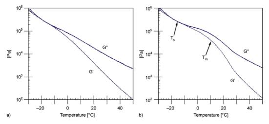
**Figure 6.** Thermal transition behaviour of storage (*G'*) and loss (*G''*) modulus in cooling (a) and heating ramp (b) of PDM-PEO-PPO-PEO-PDM-L
