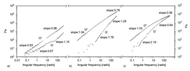
Figure 8. Frequency sweeps of a) PEO-PPO-PEO-H, b) PDM and c) PDM-PEO-PPO-PEO-PDM-H measured at 60°C
