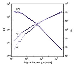
Figure 9. Frequency dependence expressed as complex viscosity ( $\eta^*$ ), storage modulus (G') and loss modulus (G'') of PDM-PEO-PPO-PEO-PDM-L. Horizontal shift factor  $a_T = 0.2468$  and vertical shift factor  $b_T = 2.039$ . Reference temperature is 35°C.
