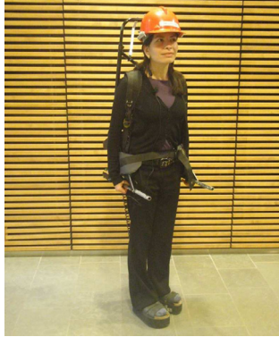
Figure 4.3: The restrictive outfit used to mimic astronaut space suit constraints consisted of wooden platform sandals, a backpack and a helmet.
