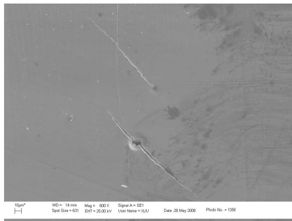
Figure 4.1: Microcracks at a surface cavity of the Ni_{50.5}Mn_{28.0}Ga_{21.5} specimen after 10.5 \cdot 10^6 magneto-mechanical cycles with 1 % p-p strain (a bright field secondary electron image).
