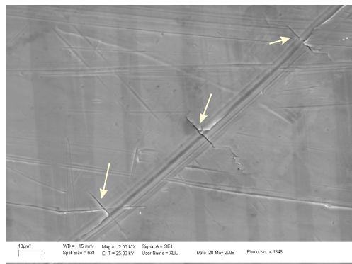
Figure 3.14: Microcracks (indicated by arrows) at a surface scratch of 10M Ni_{50.5}Mn_{28.0}Ga_{21.5} after magneto-mechanical cycling of 107 \cdot 10^6 cycles at \epsilon_a \approx 1\% . A secondary electron image (SEI).
