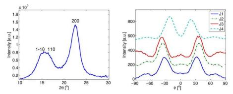
**Fig. 1.** Left: Intensities around the cellulose reflection 200 measured for the juniper pulp sheet in symmetrical reflection mode. Right: Azimuthal intensity profiles of the cellulose reflection 004 for the juniper wood samples (from top to bottom: the sample 0.5 cm from the bark to the sample 0.5 cm from the pith)
