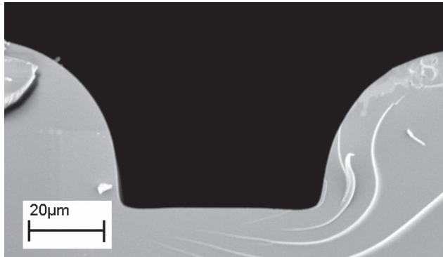
Figure 4.8. Profile of the channel embossed with the hard stamp
