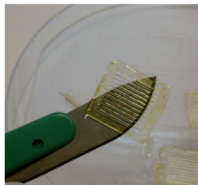
Single polymer layer detached from the PMMA
