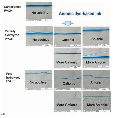
Figure 8. The cross-section optical microscopy images of polyvinyl alcohol films after 5 s self-made anionic ink absorption. The additive amount was 1 pph (cationic or anionic) or 4 pph (more cationic or more anionic).
