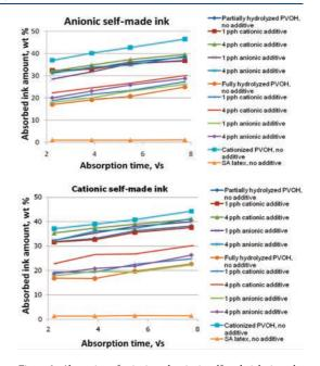
**Figure 2.** Absorption of anionic and cationic self-made inks into the PVOH and SA latex films, expressed as the weight fraction of film weight. The standard deviation of absorbed ink amount was at maximum 2 wt %, but in most cases, it was about under 1wt %.
