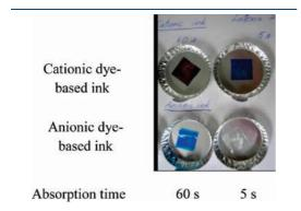
Figure 6. The self-made cationic and anionic dye-based ink absorption into the anionic latex film after 60 and 5 s absorption times, respectively.
