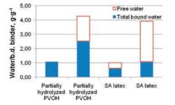
Figure 3. The water type (bound versus unbound) in PVOH and SA latex films, as measured with DSC. The dissolving of PVOH likely has some effect on the results.
