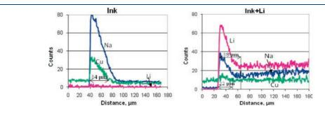
Figure 5. The location of ink (Cu and Na) and water (Li) in the PVOH film layer. Measured with ToF-SIMS.
