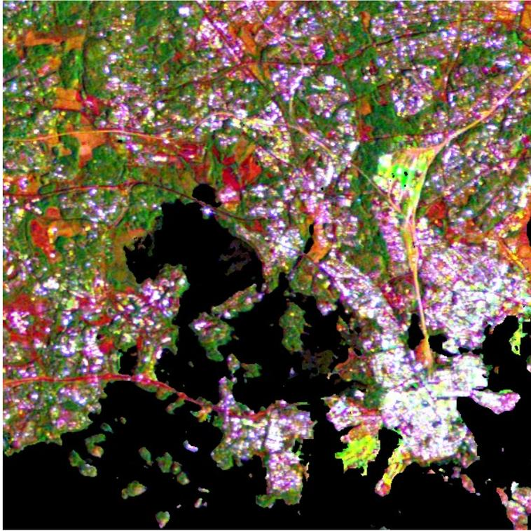
**Figure 3.** An example of a multitemporal interferometric SAR dataset (from I; SAR data © M. Engdahl and ESA AO3-277). The channels of the colour image: temporal average of Tandem coherence images in red, temporal average of backscatter intensity images in green, and average of two long-time coherence images in blue. The figure shows a 12 km × 12 km subarea of the dataset.
