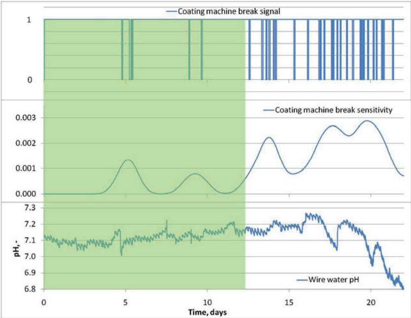
**Figure 31** Relations between coating machine's runnability and paper machine's chemical stability. The part with color presents the period with good runnability. Break sensitivity is calculated from the break signal according to equations 1 and 2. *Paper V*.
