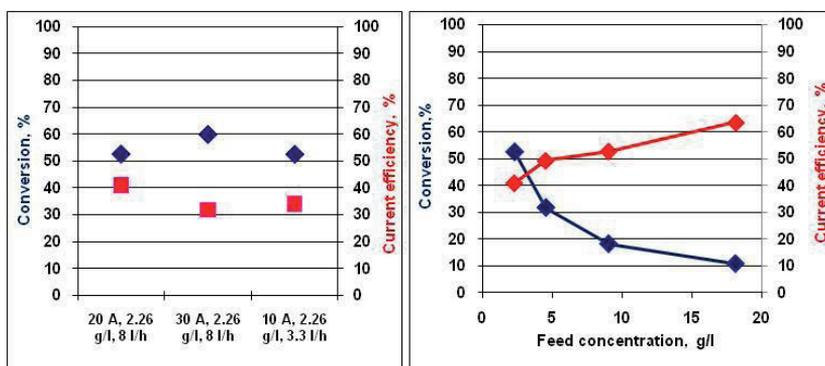
**Figure 34** Conversion and current efficiency at different operating conditions (left) and the effect of NaCl feed concentration on conversion and current efficiency (right), current 20A and flow rate 8l/h.
