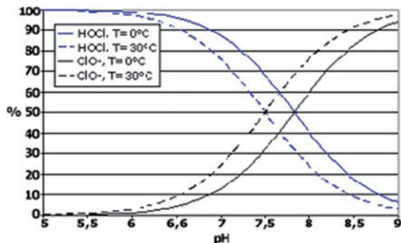
**Figure 9** Dissociation of hypochlorous acid at various pH values (<http://www.electrolyseur.com/images/hypochlorite.jpg>)
