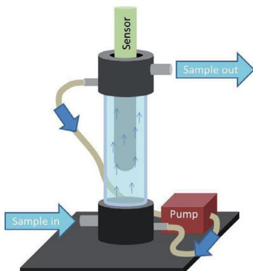
**Figure 11** Flow chamber with auto-stirring system.
