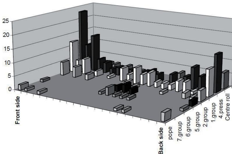
**Figure 3** The location of web breaks during a six months follow-up study at a magazine paper machine in Finland (Hokkanen 1996).
