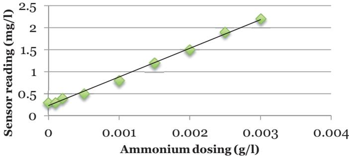
**Figure 18** Response of ISE ammonium measurement (YSI Professional Plus) to ammonium dosing into process water sampled from a paper machine.
