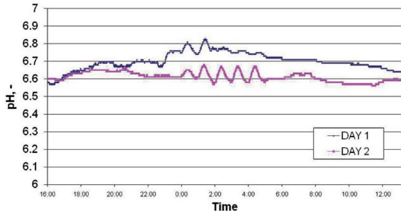
**Figure 26** pH in the water removal chest during felt washing measured with YSI 556MPS. *Paper III.*
