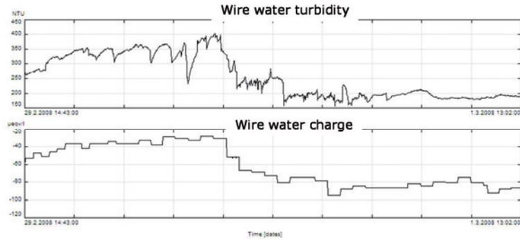
**Figure 23** Online turbidity (measured with YSI 6920V2) and charge (with Mütek PCT20) measured from a flow after the wire pit. *Paper III.*
