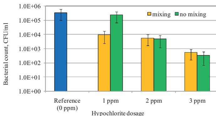
**Figure 38** Effect of mixing on the clear filtrate biocide treatment efficiency with electrochemically formed hypochlorite. Error bars represent deviation between 3 parallel platings. Mixing was applied with a three-blade mixer with rotation speed 180rpm. *Paper II.*
