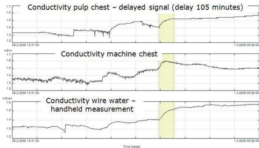
**Figure 25** Detection of process delay based on handheld devices (YSI 556MPS). Delayed signal is generated in process analysis software by shifting the time axis. *Paper III.*
