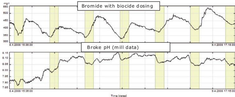
**Figure 20** Biocide feeding generates chemical variations in the process. Bromide concentration was measured with YSI Professional Plus. Colorings present the dosing of biocide. *Paper III.*
