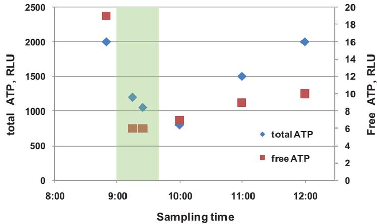
**Figure 17** ATP (free and total) measurements on wire water to monitor the effect of biocide performance. Coloring presents the dosing of biocide (hypochlorite was added for 40 minutes time). *Paper IV*.
