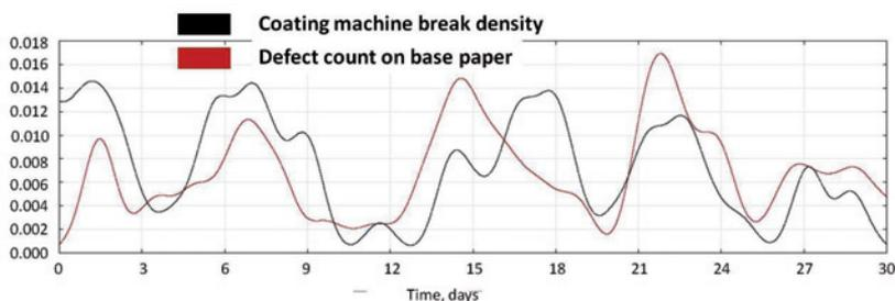
**Figure 32** Correlation between base paper defects and coating machine runnability. Break density and defect count are calculated according to equations 1 and 2. *Paper V*.
