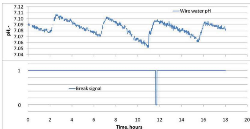
**Figure 30** Occurrence of web breaks at PM due to a pH shock generated by the biocide dosing. *Paper V.*
