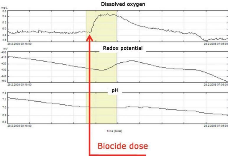
**Figure 29** The effect of oxidative biocide feed on dissolved oxygen, redox potential, and pH measurements (measured with YSI 6920V2). A coloring presents the dosing batch of the biocide. *Paper III.*
