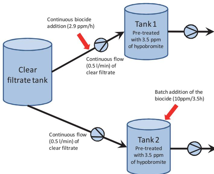
**Figure 12** Trial setup for the determination of the effect of dosing mode. Flow rates of the pumps were synchronized so that the clear filtrate levels in the tanks 1 and 2 were constant.
