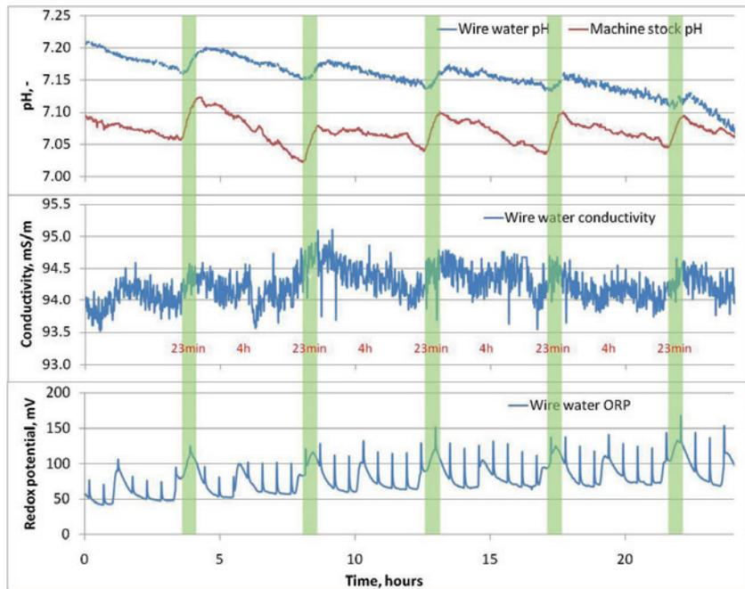
**Figure 28** Chemical variations in the short circulation due to the biocide addition. Colorings present the batch-wise added biocide dosing. *Paper V.*
