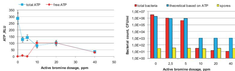
**Figure 22** Optimization of biocide dosage with a portable ATP luminometer. Biocide was dosed to fine paper machine's clear filtrate. Viable bacteria were calculated on the basis of intracellular ATP, which was estimated by subtraction of free ATP from total ATP content. ATP values are averages of at least three measurements. *Paper IV*.
