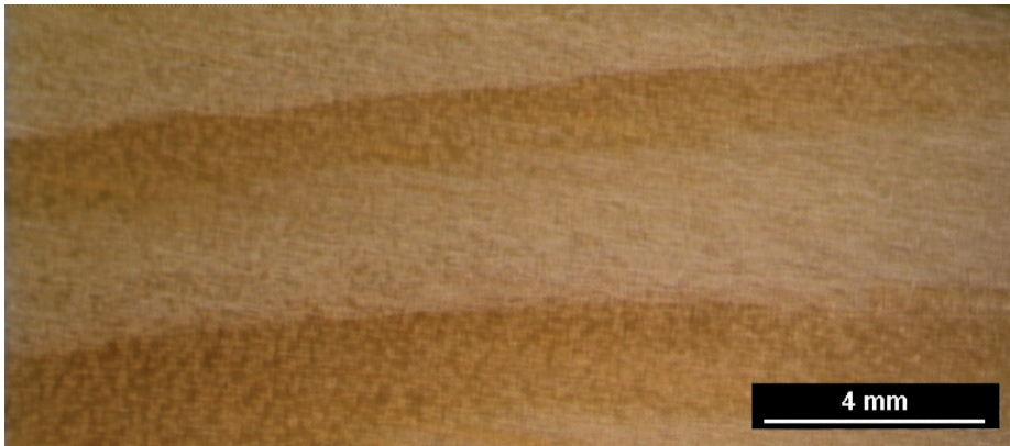
Fig. 19 Surface of Scots pine sapwood, densified using friction (Paper VI).
