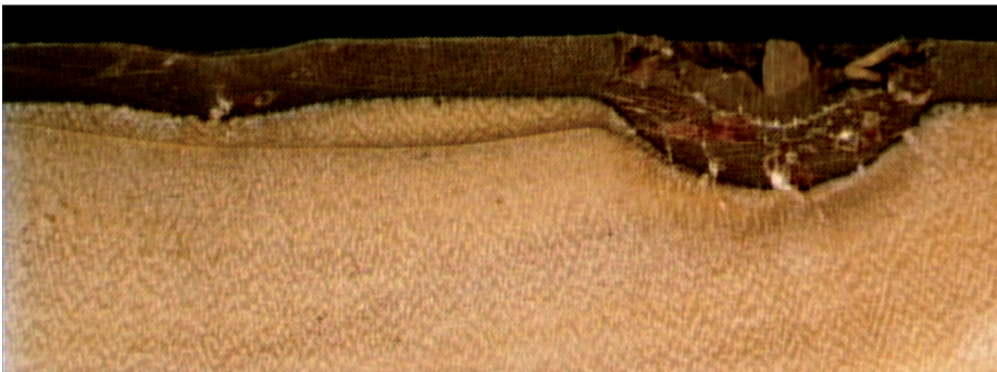
Fig. 7 Low density hybrid poplar laminated with high density VTC wood. Two different types of penetrations presented, using low (left side) and high (right side) forces.
