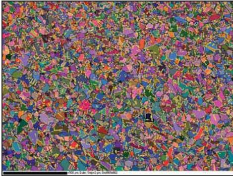
**Figure 101.** Euler map of sample 4D. Twin boundaries are seen as yellow. Length of the scale bar is 500  $\mu\text{m}$ . (Savolainen et al. 2008)
