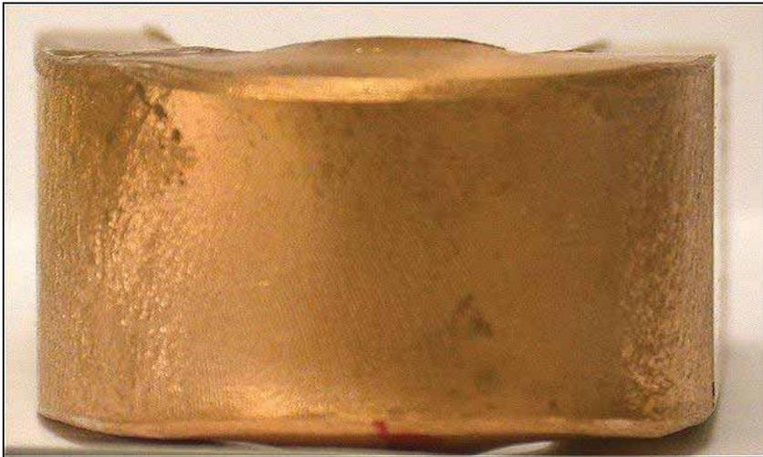
**Figure 131. Bend test specimen of Cu-OF (Savolainen et al. 2004).**
