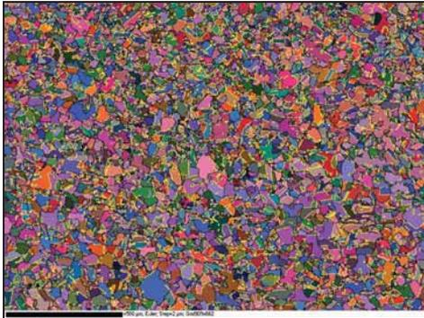
**Figure 93.** Euler map of the reference sample 1D. Twin boundaries are shown as yellow. Length of the scale bar is 500  $\mu\text{m}$ . (Savolainen et al. 2008)
