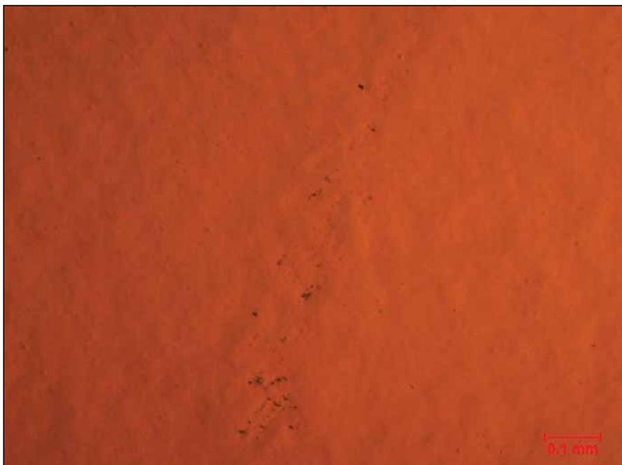
Figure 125. A detail of the entrapped oxide particle line in a 50 mm thick Cu-OFP FSW weld shown in Figure 121. (Savolainen et al. 2012b)
