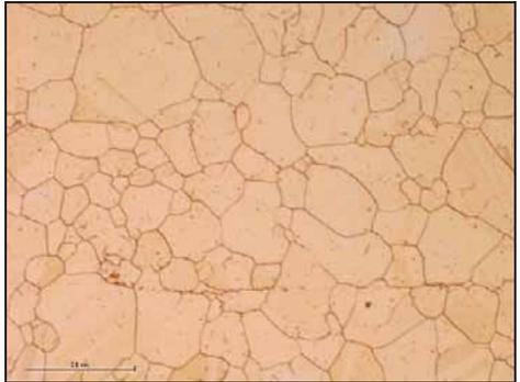
**Figure 82. Detail of hydrogen annealed sample FSW welded with oxide removal and shielding gas. Length of the scale bar is 0.5 mm. (Savolainen et al. 2008)**
