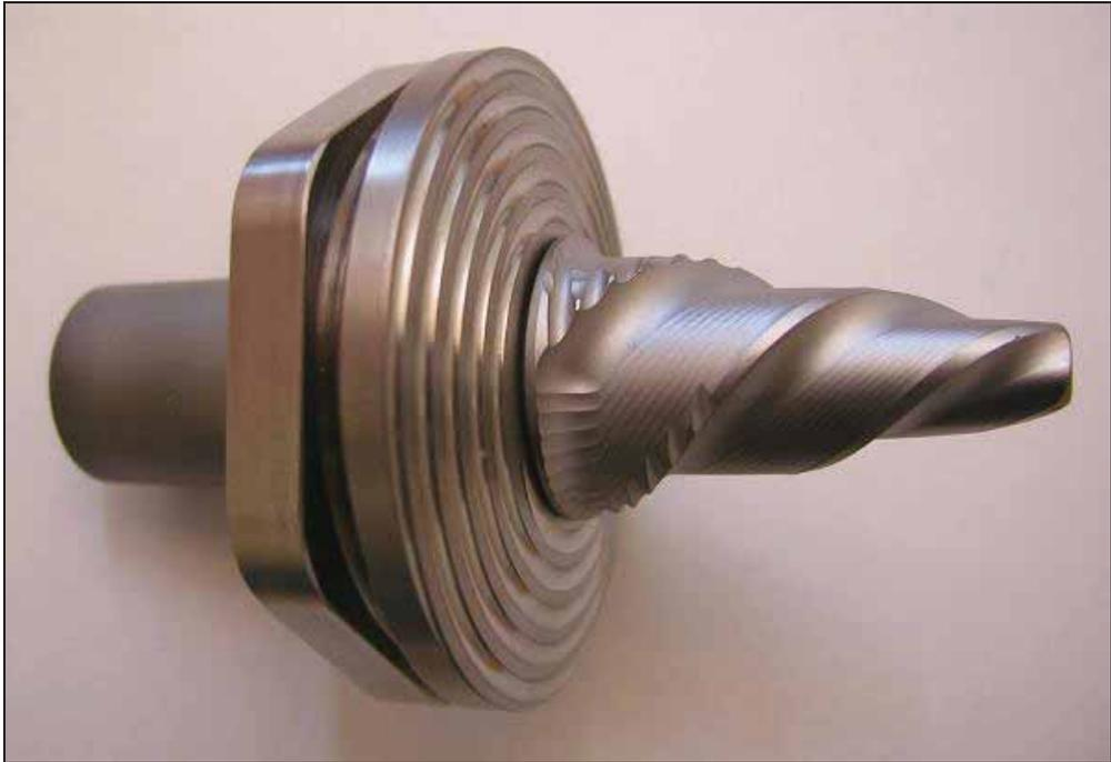
**Figure 11. The tool currently used by SKB for FSW of 50 mm thick Cu-OFP to be applied for manufacturing spent nuclear fuel canisters. The tool has a probe with a complex triflute design and a CS4 shoulder. (Cederqvist 2011)**
