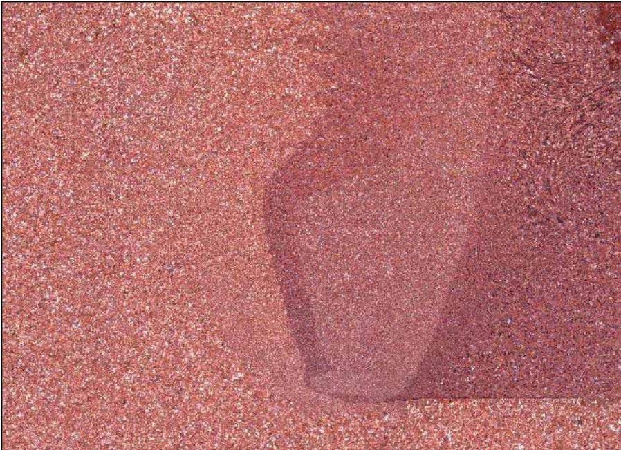
**Figure 45. Many microstructural zones are visible in the transverse cross-section of a 50 mm thick Cu-OFP FSW weld. Forged lid (on the left, retreating side) and extruded tube (on the right, advancing side) are the base materials. (Savolainen et al. 2010)**
