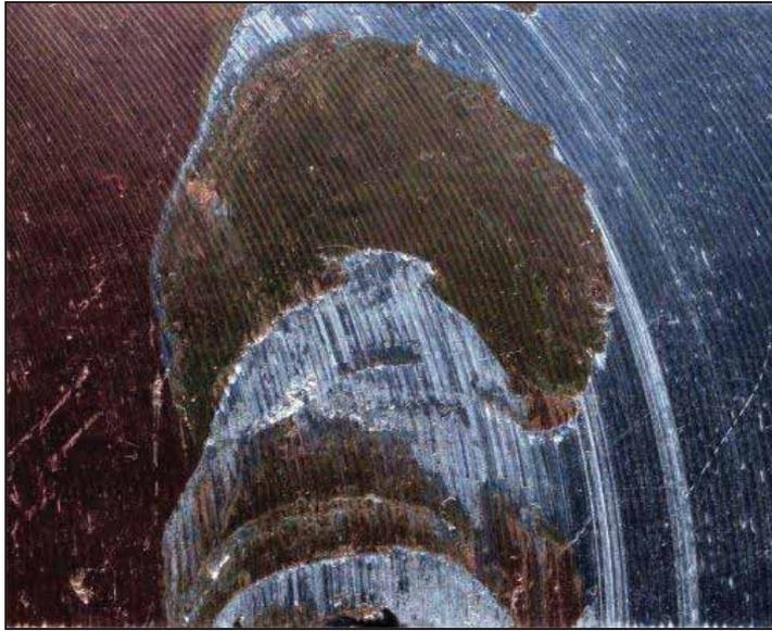
**Figure 70. The Cu/Al dissimilar metal FSW weld 2004-10-27A (Table 7). Welding parameters were 750 rpm and 150 mm/min.**
