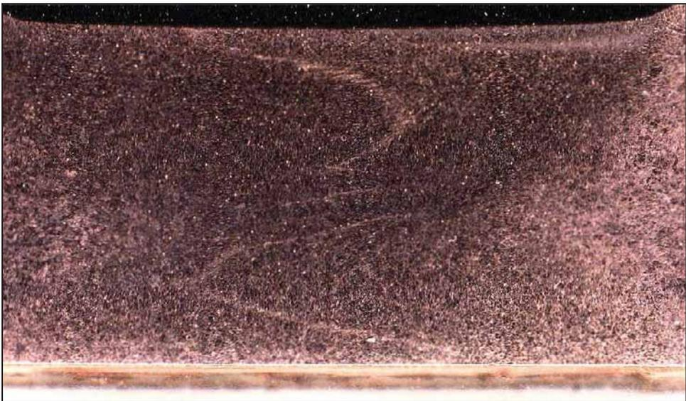
**Figure 31. Entrapped oxide particle lines in a double-sided Cu-OF FSW weld.**
