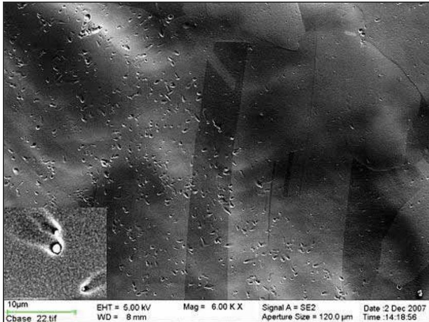
Figure 54. SEM image showing the origin of the contrast in the FSW weld marked by C in Figure 53. Weld is on the right and base material on the left. EDS study revealed that the features on the left are  $\text{Cu}_2\text{S}$ . The insert shows  $\text{Cu}_2\text{S}$  precipitates of the base material and their “tail” in greater detail (Saukkonen et al. 2008)
