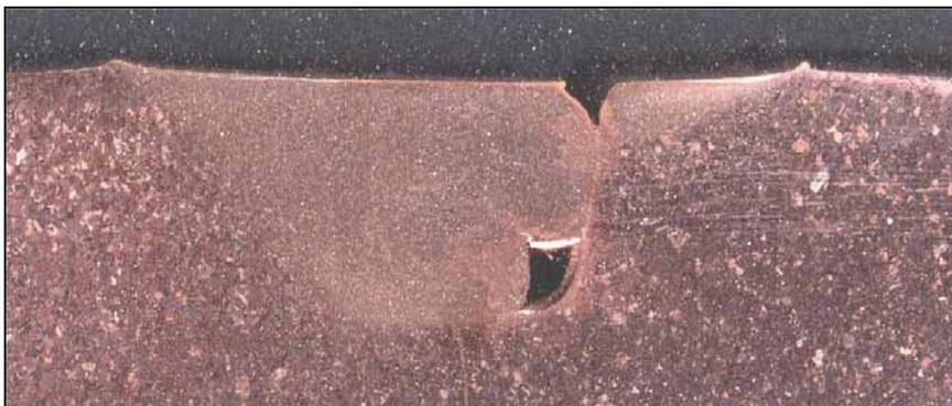
**Figure 28. Similarity in the formation of surface-breaking and sub-surface voids in a copper FSW weld.**
