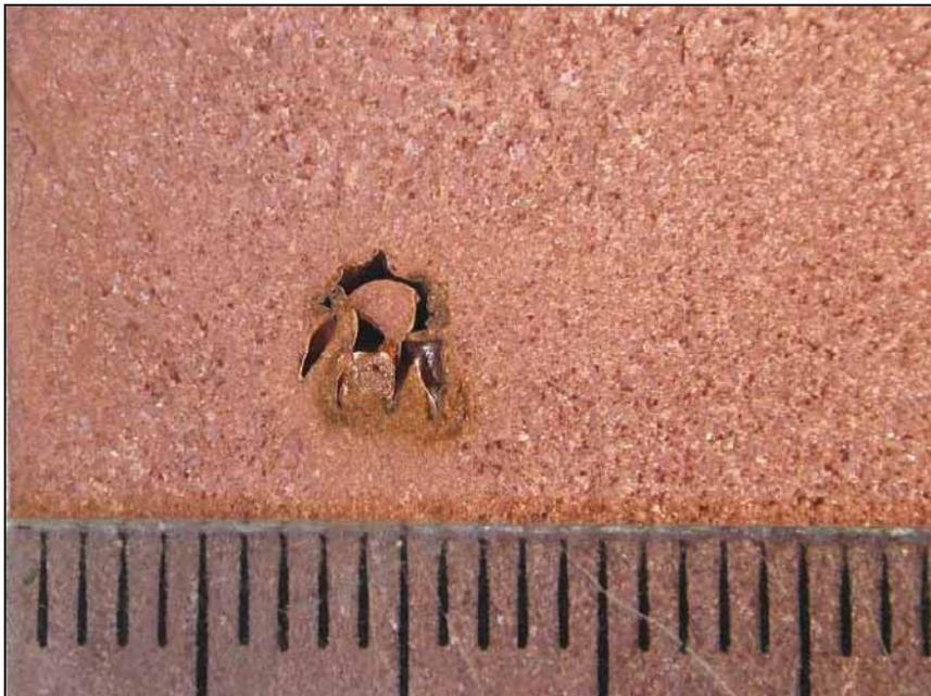
**Figure 29. Void in the upper part of a 50 mm thick copper FSW weld (SKB 2005).**
