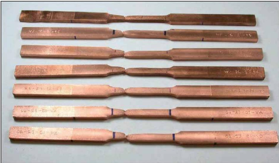
**Figure 115. Cu-DHP tensile test specimens. The base material specimen is on the top. The FSW welds are located at the centre of the gauge lengths. The fracture locations in the HAZ/base material region of the FSW welds can be seen. (Savolainen et al. 2004)**
