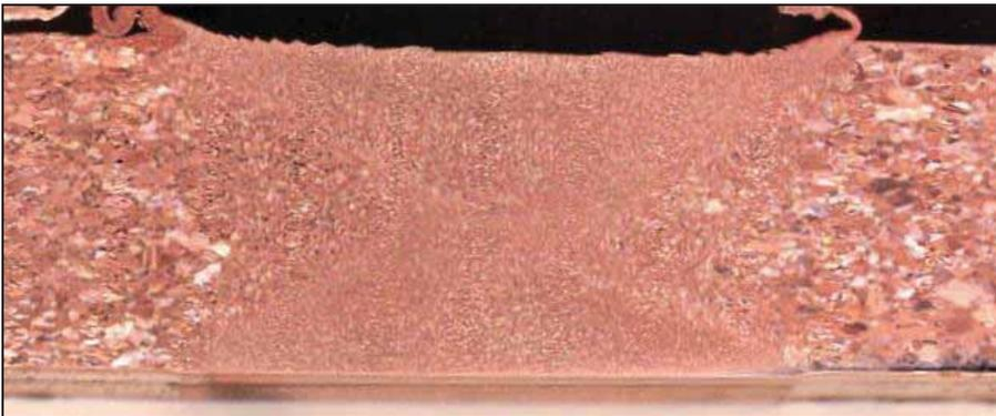
**Figure 44. Double-sided FSW weld of cold-rolled Cu-OF with 10 mm plate thickness. Smaller grain size in the weld is evident. No separate zones are readily seen contrary to Figure 45.**
