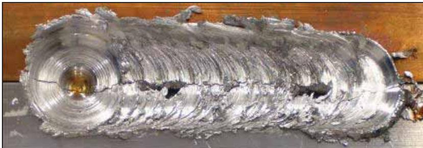
**Figure 65.** An example of a poor quality Cu/Al dissimilar metal FSW weld, 2004-10-14A (in Table 7). Aluminium was on the advancing side, no tool displacement. Welding parameters were 1000 rpm and 100 mm/min. No proper joint was formed between the plates.
