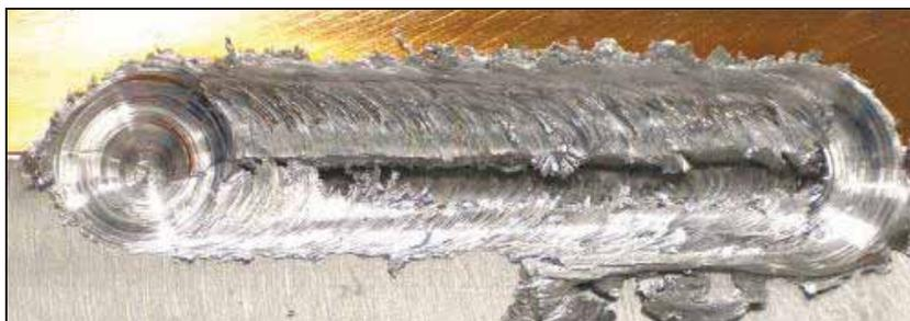
**Figure 66.** An example of a poor quality Cu/Al dissimilar metal FSW weld, 2004-10-19E (in Table 7). Tool displacement was 1.5 mm on the aluminium side. Aluminium was on the advancing side. Welding parameters were 750 rpm and 100 mm/min. It is noteworthy that with the same welding parameters, a good weld is produced when copper is on the advancing side. With aluminium on the advancing side, a large groove is formed on the aluminium side.
