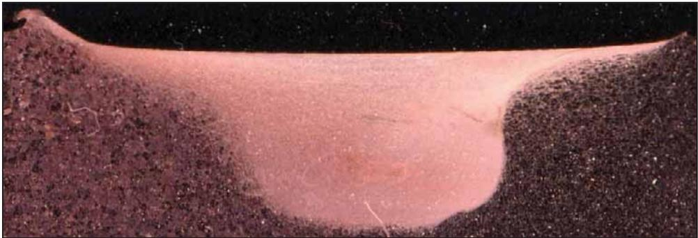
**Figure 30. LOP in a Cu-DHP weld.**
