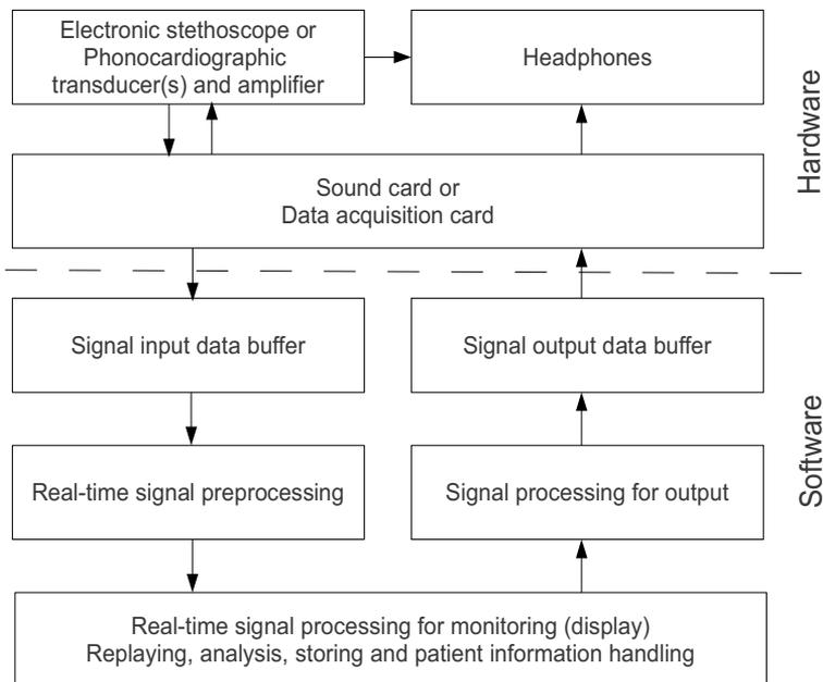
**Figure 4.2.** Block diagram of the heart sound signal processing flow in the phonocardiographic system showing the hardware/software interface (Adapted from Sikiö 1999).
