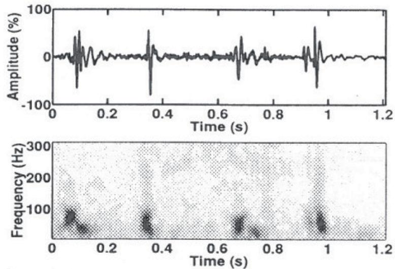
**Figure 6.1.** Phono-spectrographic presentation of two cycles of innocent vibratory murmur. For visual analysis the original signal was down-sampled from 11,025 Hz to 2,205 Hz and pass-band filtered from 50 to 300 Hz. The spectrogram is calculated using 128-point FFT and 75 % overlapping between the segments (Publication I).
