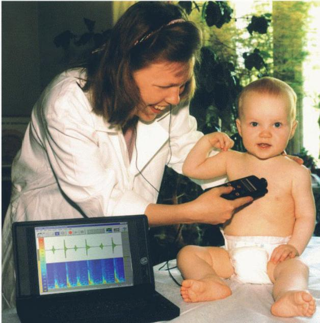
**Figure 4.1.** The phonocardiographic system developed consisting of the electronic stethoscope with headphones connected to a multimedia laptop computer
