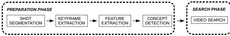
Figure 4.7. Processing stages of a video retrieval system. Adapted from Publication VI.
