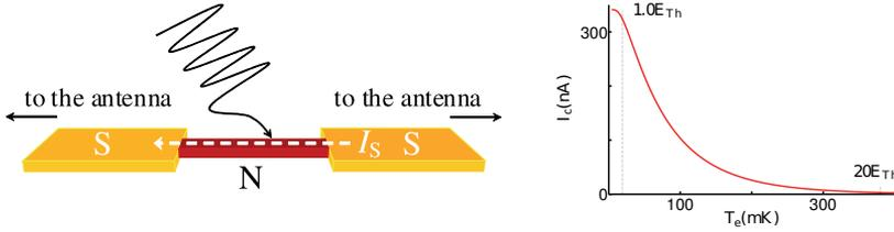
**Figure 4.3.** In the Proximity Josephson sensor external antennas couple incident radiation to the detector, composed of a proximity nanoconductor. The critical supercurrent  $I_c$  is a sensitive function of the nanoconductor electron temperature  $T_e$ .
