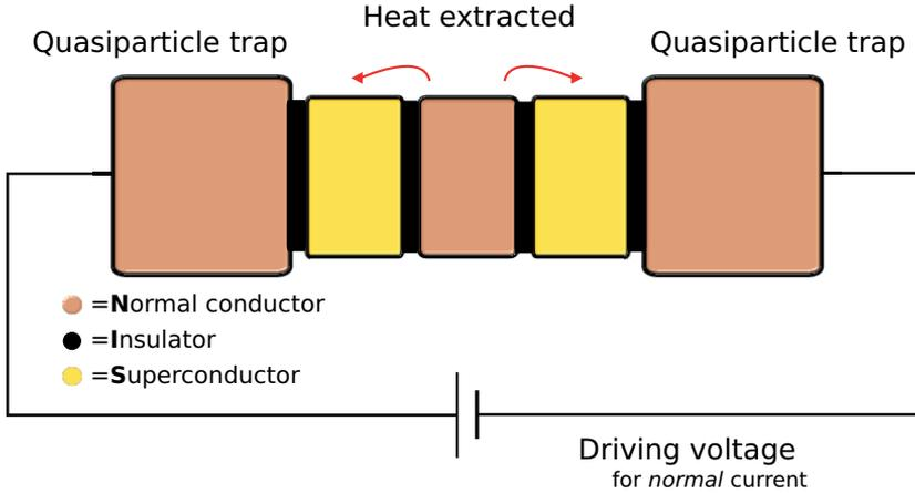
**Figure 4.4.** SINIS electron cooler can be complemented by an additional layer of N electrodes which act as quasiparticle traps, i.e., as perfect reservoirs which aim to remove energy from the superconductors.
