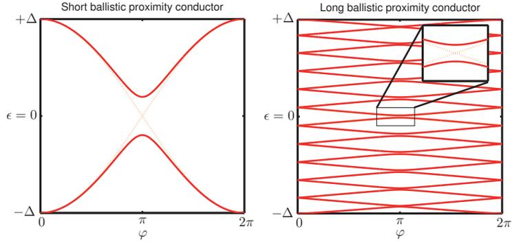
**Figure 2.5.** Subgap energy spectrum in short and long ballistic proximity conductors as a function of phase difference  $\varphi$ . The dotted line shows the spectrum in the ideal case when the N-S interface is completely transparent and the solid line corresponds to a case where there is some normal scattering at the interface.
