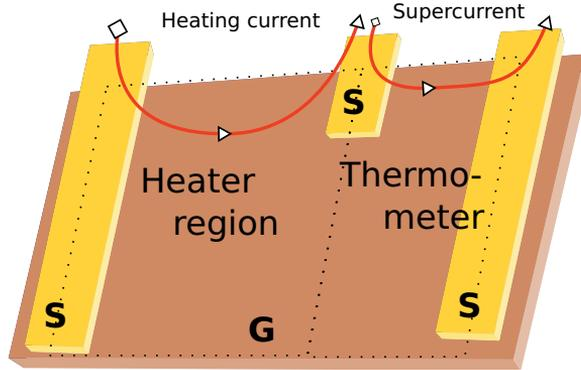
**Figure 4.2.** Graphene thermometer is composed of a heater and a thermometer junction. Superconducting leads (S) deposited on top of graphene (G) allow both heating normal current and probing supercurrent to be run through the device.
