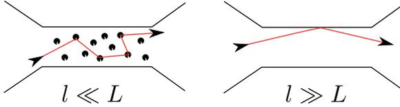
**Figure 2.3.** Diffusive and ballistic conductivity for a nanoconductor with length  $L$  and elastic relaxation length  $l$  which is roughly of the same order as the distance between individual elastic scattering events.
