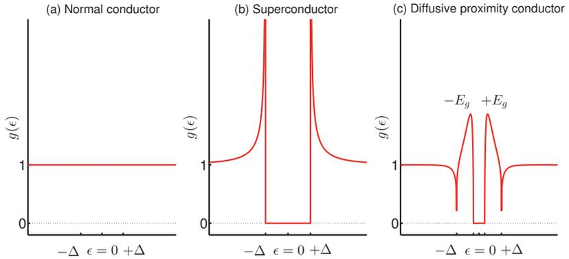
**Figure 2.4.** Density of states in a normal conductor, in a superconductor and in a specific realization of a diffusive proximity conductor (at the midpoint), all normalized to the density of states of the same system in the normal state so that  $g(\epsilon) = N(\epsilon)/N_F$ .
