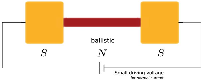
**Figure 4.5.** In an ideal ballistic SNS nanoconductor scattering is absent both inside the nanoconductor and at the N-S interfaces. We study, how departure from this ideal affects transport at the low-voltage limit.
