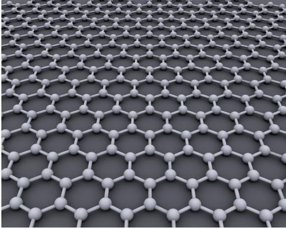
**Figure 4.1.** Graphene lattice is shaped like a honeycomb with bonds of length 0.14 nm connecting individual carbon atoms
