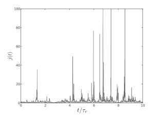
FIG. 10. (Color online) Three simulated realizations of current in an overheated SET at  $\nu$ =0 and  $\mathcal{D}$ =3.3. The average current (for  $\mathcal{D}$  $\rightarrow$ 0) is j $\approx$ 1.7.
