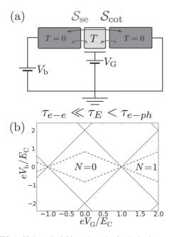
FIG. 1. (Color online) (a) A schematic of a single-electron transistor, biased by voltage  $V_b$ . The charge on the island can be tuned with the gate voltage  $V_G$ . (b) Coulomb diamonds in a symmetric SET. Dashed line shows the threshold voltage  $V_C$ . Changing the gate voltage has the effect of changing  $V_C$ .
