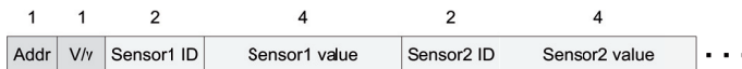
Figure 3.4. SSI sensor data response 'V' message. Addr is the device address, one byte, followed by the message type 'V' or 'v'. Either only values of the requested sensors are sent (if SensorIDs are listed in the request command 'R' or 'r') or all the sensor values requested are sent (if no SensorIDs listed).
