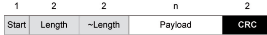
Figure 3.6. SSI/UART message format. Start byte indicating beginning of message is 0xFE. Length and ~Length are length and bitwise not of length of message payload with optional CRC.
