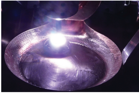
Figure 3.23. The arc melting of a BMG alloy ingot on top of the water-cooled copper hearth. On the right is the tip of the manipulator used to flip the ingot upside down between melting runs. The mould orifice and the melt pouring nozzle leading to it can be seen behind the arc (thesis Paper IV).
