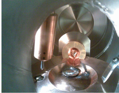
Figure 3.33. Inside view of the furnace after tilt casting. On the water-cooled copper crucible, titanium is in the small trough on the left and BMG alloy was poured into the mold.
