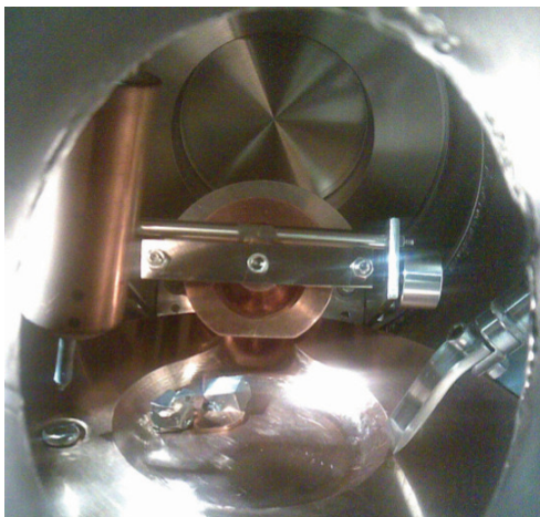
Figure 3.27. Preparing to ignite arc melting arc. The arc is always ignited to the titanium getter (under the electrode tip). In titanium gettering the highly reactive titanium is melted to remove oxygen impurities from the chamber atmosphere.
