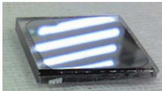
Figure 5.10. Zr-based BMG alloy deposited on a polymer substrate.
