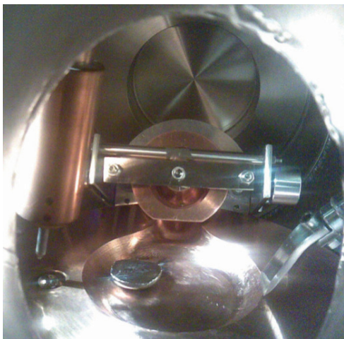
Figure 3.31. Flipped BMG ingot. The ingot was flipped without breaking the vacuum by moving it with the electrode to the right side of the trough, where it could be easily flipped with the manipulator tip.
