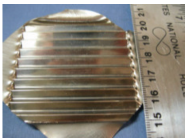
Figure 4.6. A thermoplastically compression molded nominal composition Zr_{44}Ti_{11}Cu_{10}Ni_{10}Be_{25} metallic glass plate [27].
