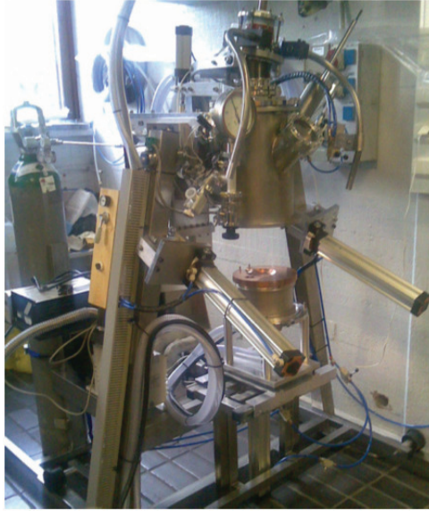
Figure 3.22. The combined arc melting and casting furnace, with chamber open.
