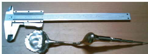
Figure 3.35. Tilt and suction cast specimen. Slow pouring left a large 'skull' on the cold copper crucible.
