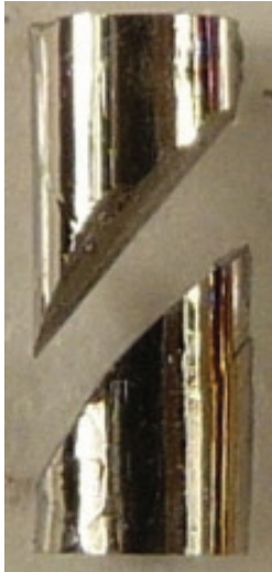
Figure 2.8. An example of a typical fractured nominal composition Zr_{55}Cu_{30}Al_{10}Ni_5 test specimen. Two shear bands can be seen, but often only one dominant shear band forms.
