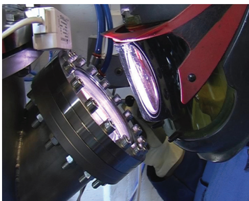
Figure 3.32. Arc melting in practice. The pneumatic valve in the middle of the picture is used to adjust the height of the electrode inside the chamber.
