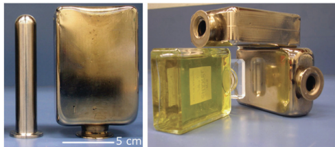
Figure 4.4. A blow molded nominal composition Zr_{44}Ti_{11}Cu_{10}Ni_{10}Be_{25} metallic glass bottle [27].
