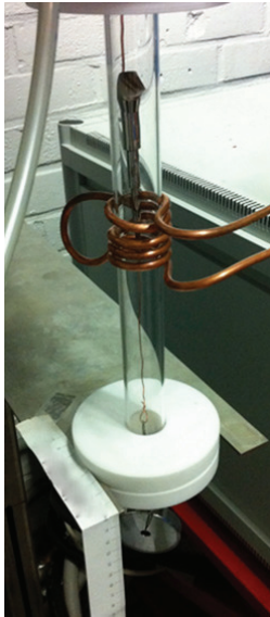
Figure 4.9. The constructed wire drawing apparatus (thesis Paper V).
