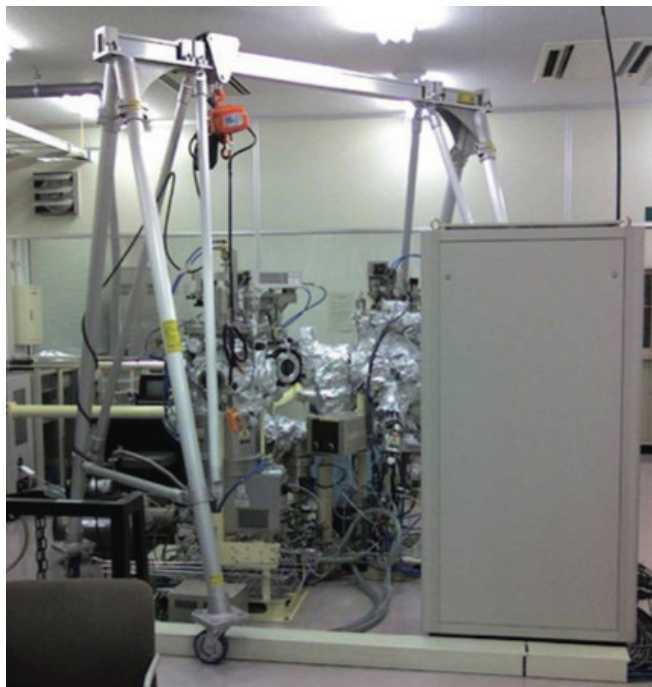
Figure 5.6. The UHV magnetron sputtering furnace used. The aluminum foil wrapping is for UHV baking the chamber, which is necessary after disassembly to achieve UHV conditions.
