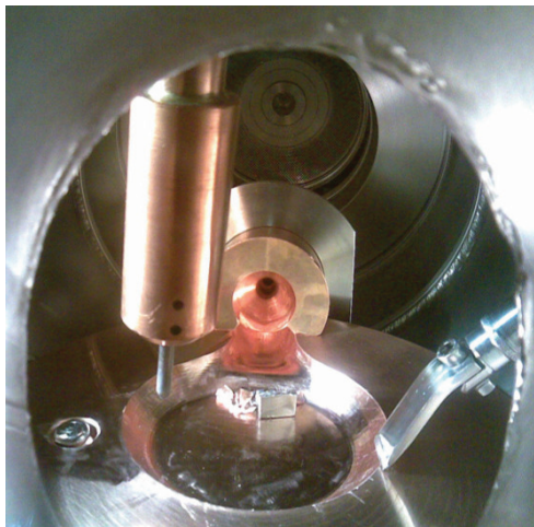
Figure 3.26. High-vacuum pumping in progress. Turbo-molecular pump rotor is spinning behind the mold.
