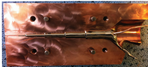
Figure 3.34. Typical mold filling with tilt and suction casting. This is the same mold shown in figure 3.4, now with better filling probably mostly due to the use of suction in the casting. This specimen also has some cast-in copper wires for an experiment that will be covered in chapter 4.
