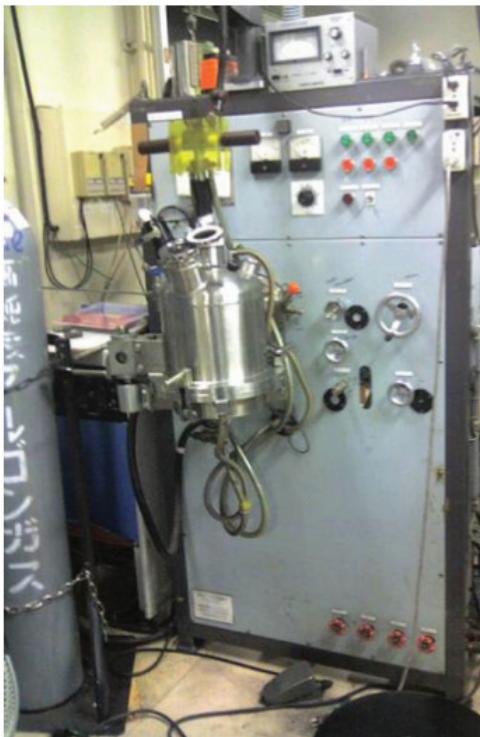
Figure 3.8. Water-cooled copper crucible arc melter used for alloying.
