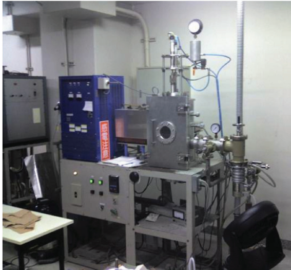
Figure 3.11. Induction casting furnace. The piston on top of the furnace moves the V-shaped quartz crucible from heating position inside the induction coil to direct contact with the copper mold orifice, when the large black button on the front of the machine is pressed.
