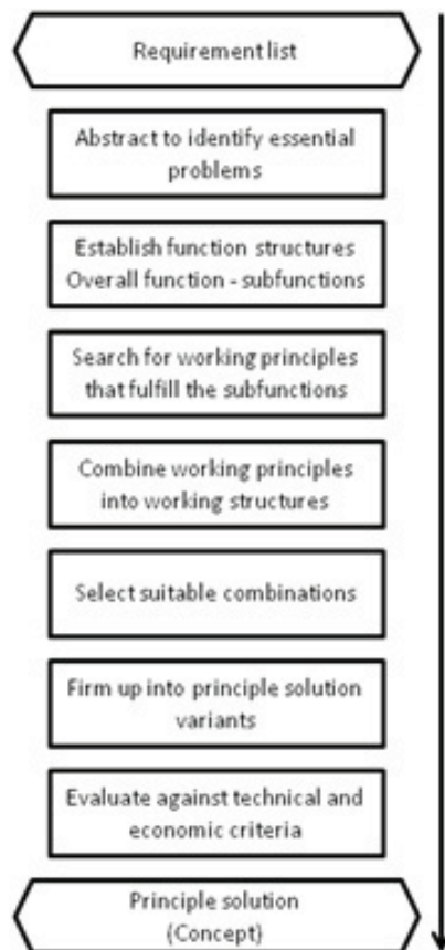
Figure 2.2. The conceptual design phase (Pahl and Beitz, 2007)
