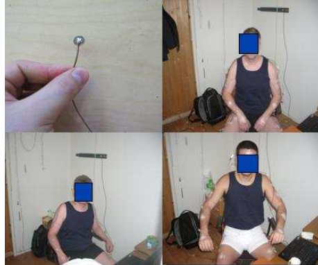
Figure 5 The used thermocouple sensor and part of the subjects after attaching the sensors at Room 2
