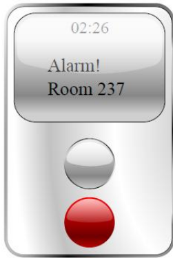
Fig. 8 Outline of a simple localization tag. The tag includes a couple of buttons and a screen for communication.
