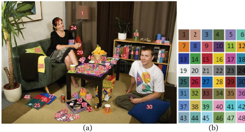
Figure 14. A test image scene with embedded color patches (a) and the colors of the patches (b) [56].
