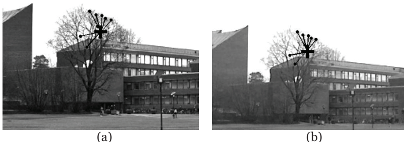
Figure 31. The center points of the correspondence areas from the reference image (a) and test image (b) are approximated by calculating the mean point of the vector heads from the correspondence feature points. The lines denote the vectors whose lengths and directions are calculated from the reference image. The points denote the correspondence-feature points. The crosses denote the correspondence-area centers.
