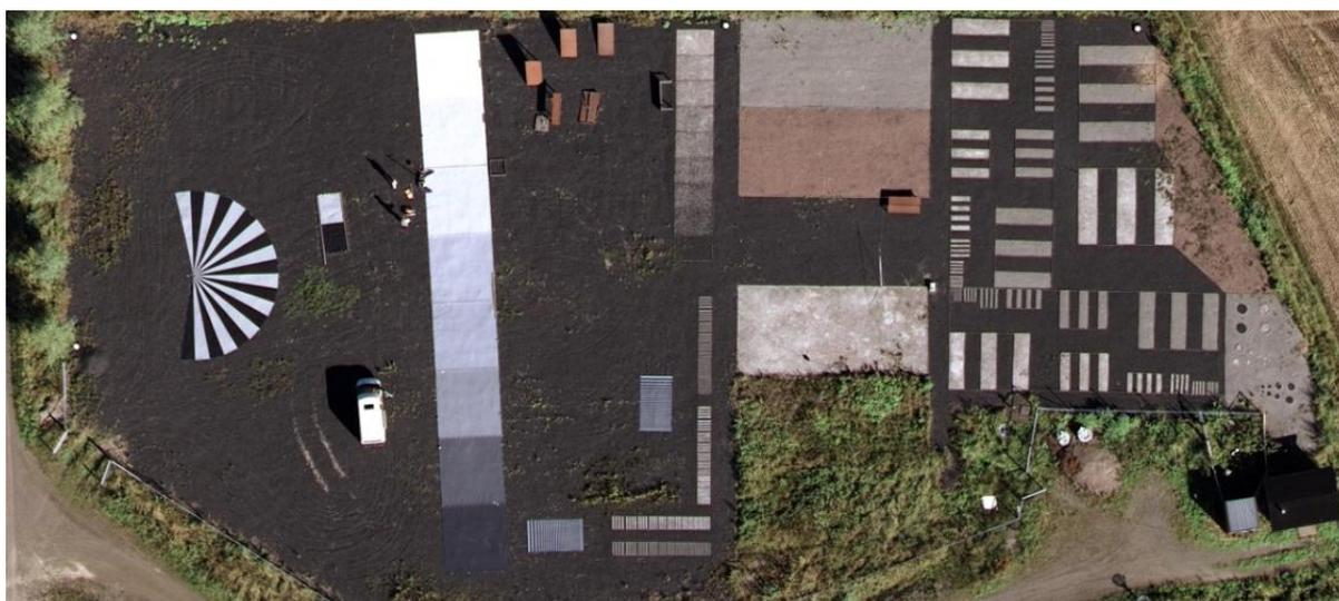
**Figure 6.** Metsähovi image quality test field in 2005 with all eight portable reference tarps installed in the form of grayscale (from **I**).
