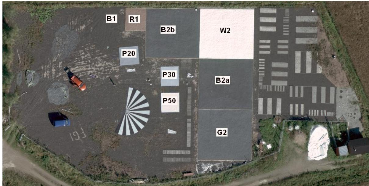
**Figure 7.** The modernized Metsähovi image quality test field in 2008 during the 1.9.2008 DMC campaign. For abbreviations, see Table 3 (from **II**).
