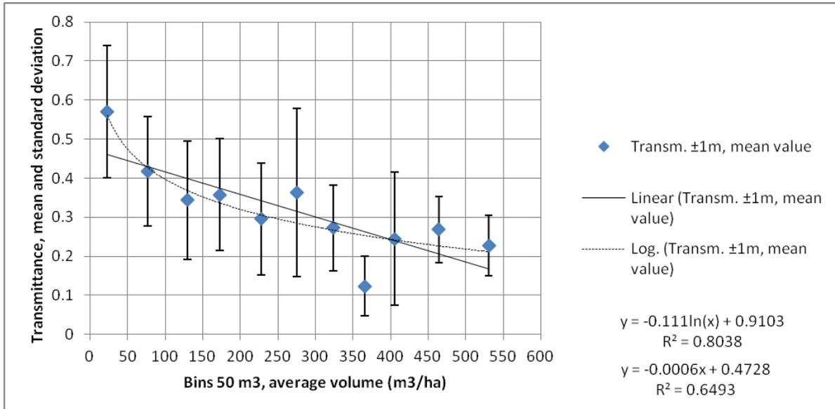
Figure 4.3. Transmittance through the canopy to the ground as a function of stem volume. Ground tolerance level  $\pm 1.0$  m.
