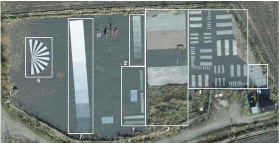
Figure 4.6. The Sjökulla test field before the renovation of areas 2) and 3). 1) Permanent dense spatial resolution target, 2) Permanent grey scale, 3) Permanent large reflectance areas, 4) Sparse resolution bar target, 5) Permanent circular targets, 6) Portable Siemens star, 7) Portable grey scale/brightness target.
