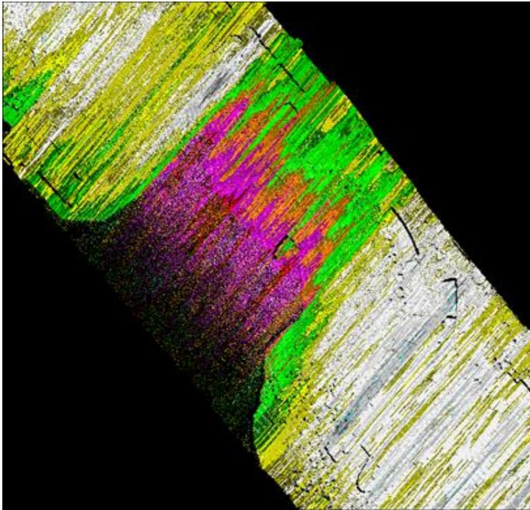
Figure 5.1. The image shows Leica ALS50II AGC's value changes in Kivenlahti Espoo caused by the water area in the middle of the image. The flying altitude was about 500 m and the swath width was about 360 m.
