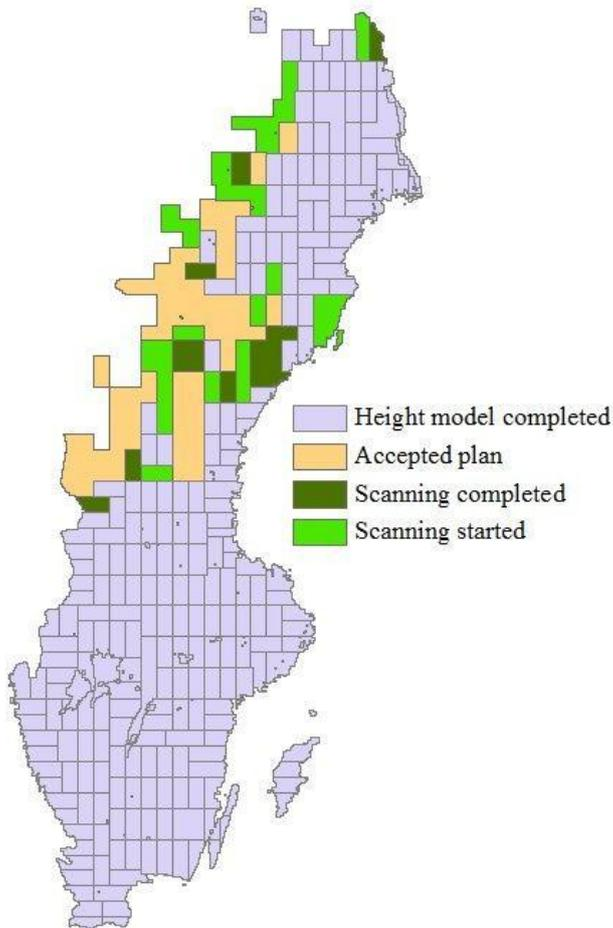
Figure 2.2. The status of the nationwide ALS in Sweden on November 8, 2012 (Lantmäteriet 2013). The scanned areas include the new height model areas (blue) and scanning-completed areas (dark green). The fell areas along the western border have a low scanning priority.
