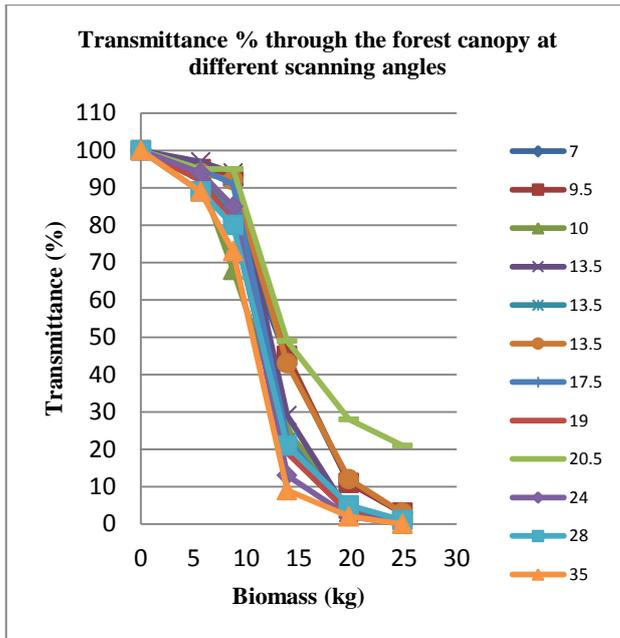
Figure 4.2. Transmittance through the forest canopy at different scanning angles (varying between 7° and 35°). We stratified the scanning angles into three groups for each height. The angle value presented is the mean value of each part.
