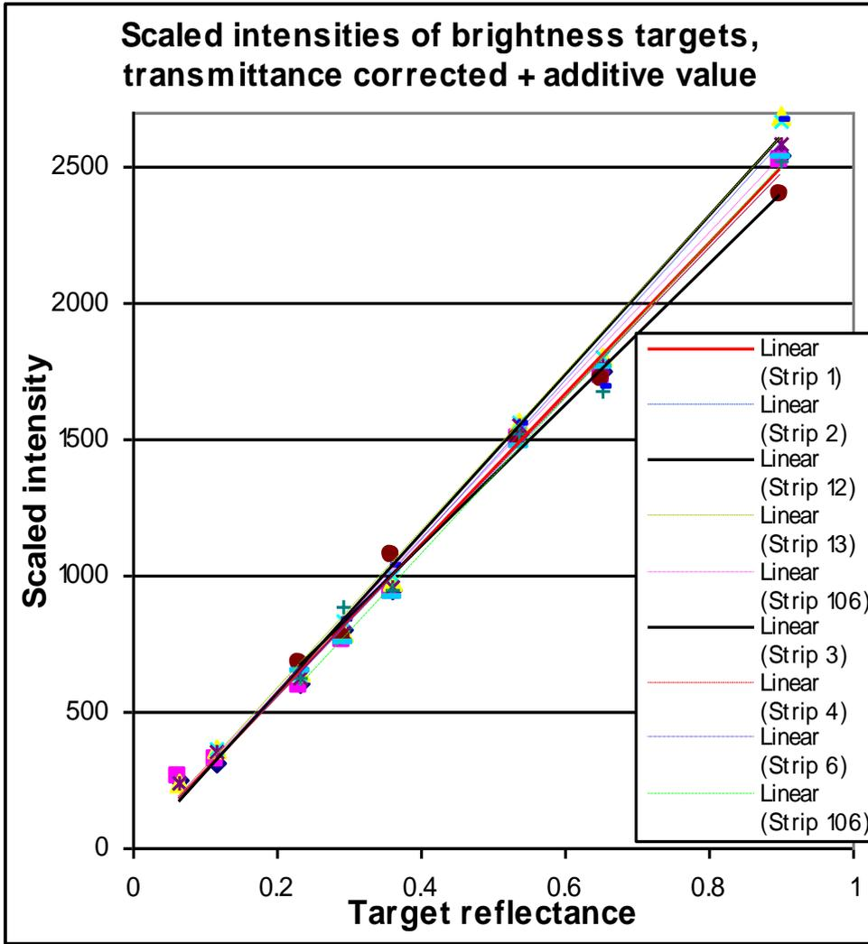
Figure 4.5. Intensity values corrected for atmospheric transmittance and additive values from regression lines. The corrected intensity values from H=200 m Strips 1 and 2, H=1000 m Strips 12, 13, 106, and H=3000 m Strips 3, 4, 6, 106 coincide very well.
