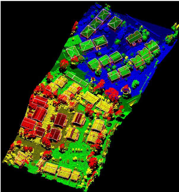
Figure 4.1. A rotated oblique view of flight strip no. 3 (first pulse) laser points and the extracted buildings.
