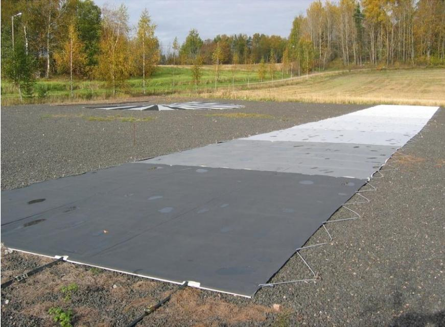
Figure 4.4. Targets at the Sjökuilla photogrammetric test field in Kirkkonummi arranged for a digital aerial camera test to represent 5%, 10%, 20%, 25%, 30%, 45%, 50%, and 70% reflectance. Photo taken on October 4, 2004 by H. Kaartinen.
