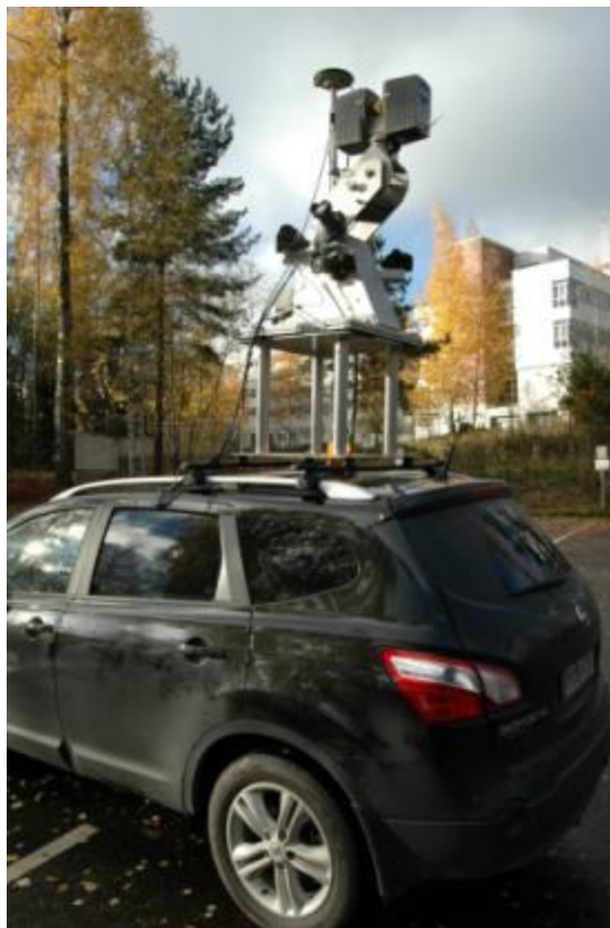
Figure 18. ROAMER system on a vehicle mount with additional imaging cluster of six Nikon D5100 cameras (Photo: H. Kaartinen, 2012).
