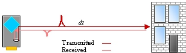
Figure 5. Principle of ToF laser ranging.
