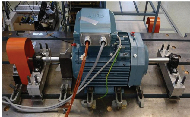
Figure 6.1. The 30 kW three-pole squirrel-cage motor used as the test-bed process.
