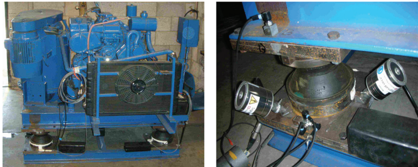
Figure 6.13. (a) The test-bed process is a marine diesel engine and a generator mounted on a raft. (b) The raft is supported by a “Smart-spring”, which consists of three inertial mass shakers and a passive damping element.
