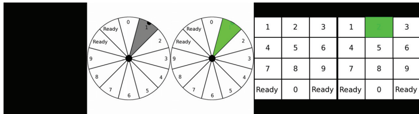
Figure 5.15. The iPad screen was used as a visual display and an input device for the touch screen interaction. When using an auditory display, the iPad screen was black (left). Circular and numpad style menus were used in the experiment.
