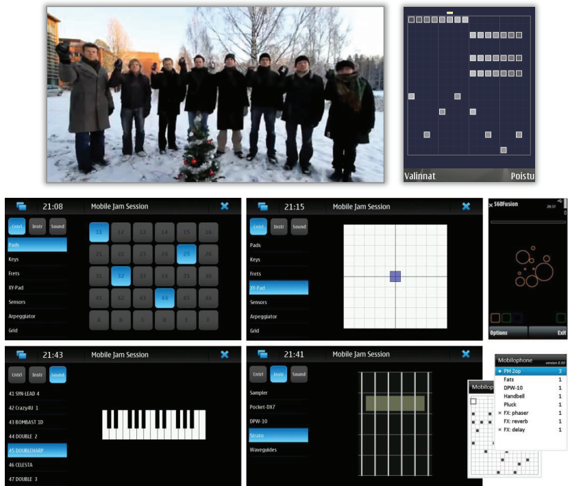
Fig. 1. Mobile audio synthesis applications implemented by the author of this thesis. The photograph shows Helsinki Mobile Phone Orchestra performing a bell choir arrangement of a Christmas song, employing accelerometer sensors and early FM synthesizer emulation.
