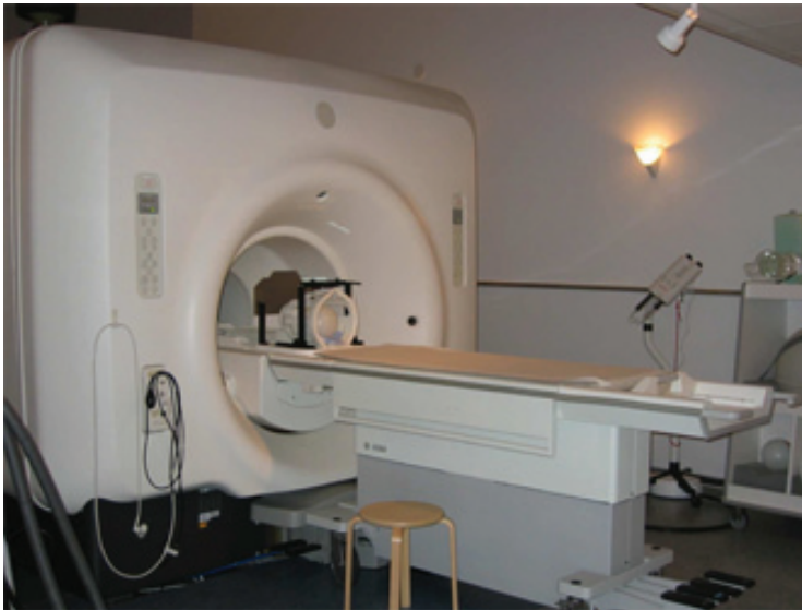
Figure 2.3. An MRI scanner at the Advanced Magnetic Imaging Centre (AMI-Centre) of the Aalto University. The subject lies down on the table in front of the scanner, placing his or her head inside the volume coil. The table is then moved into the bore of the scanner, so that the head is positioned at the very center.
