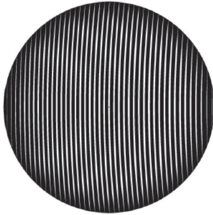
Figure 3.1. Example of a transmission-type amplitude hologram pattern. Metal is in black and slots in white. [III]
