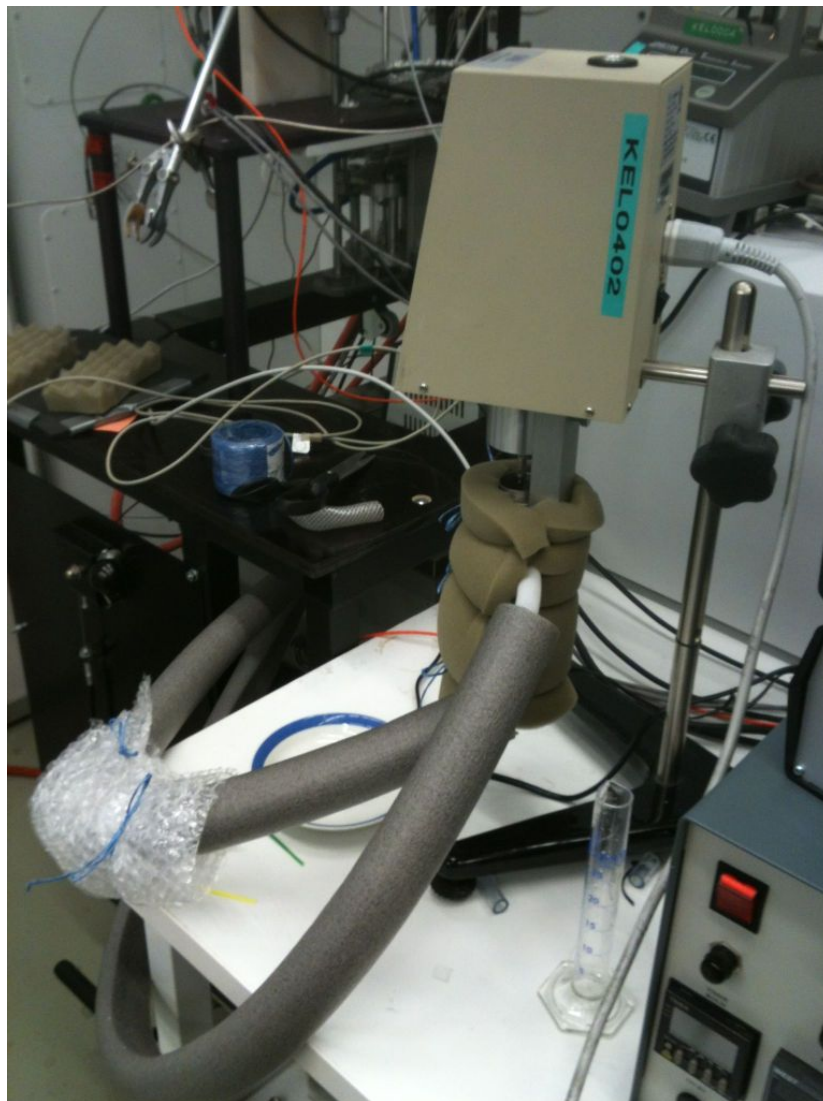
Figure 2.27. Overview of the viscosity measurement at the low temperatures
