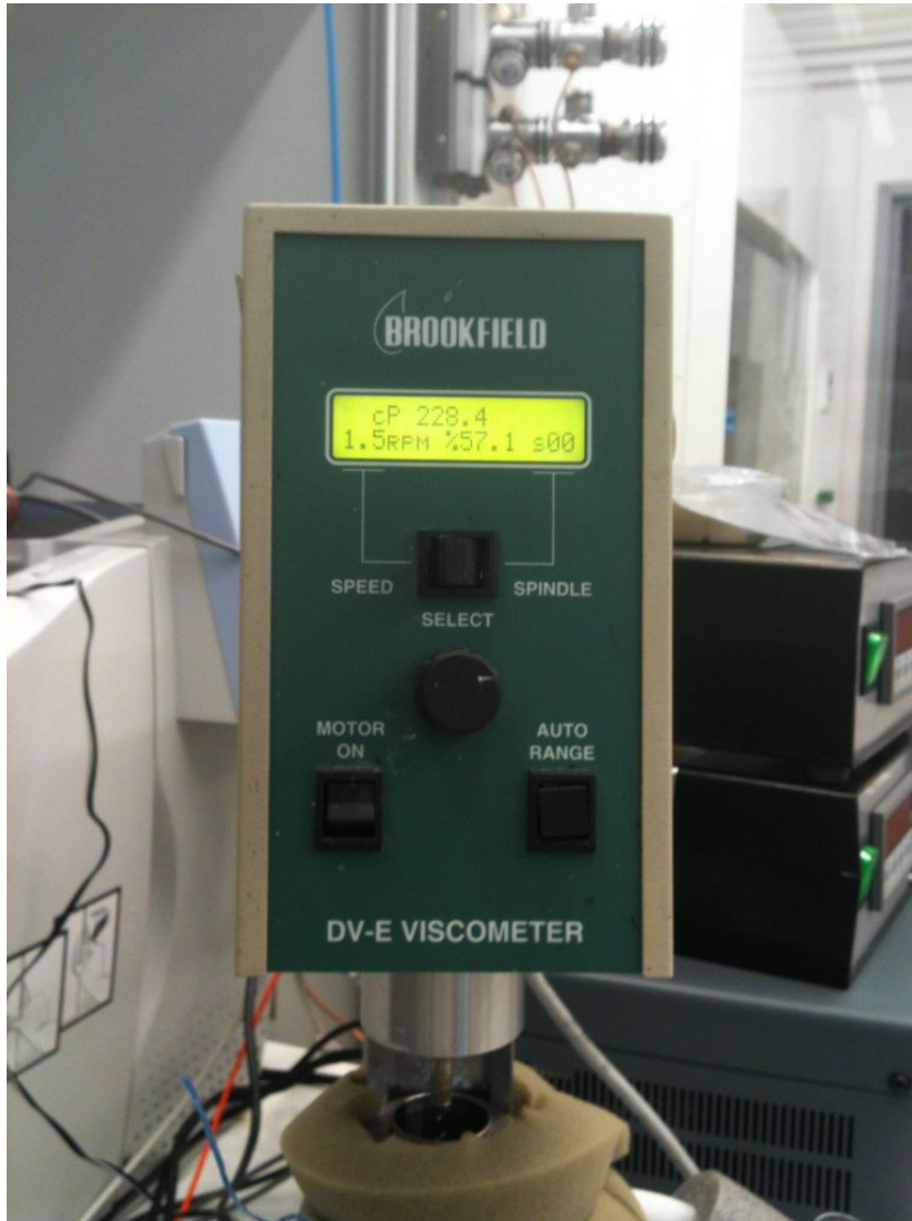
Figure 2.25. Viscometer used in the viscosity measurements
