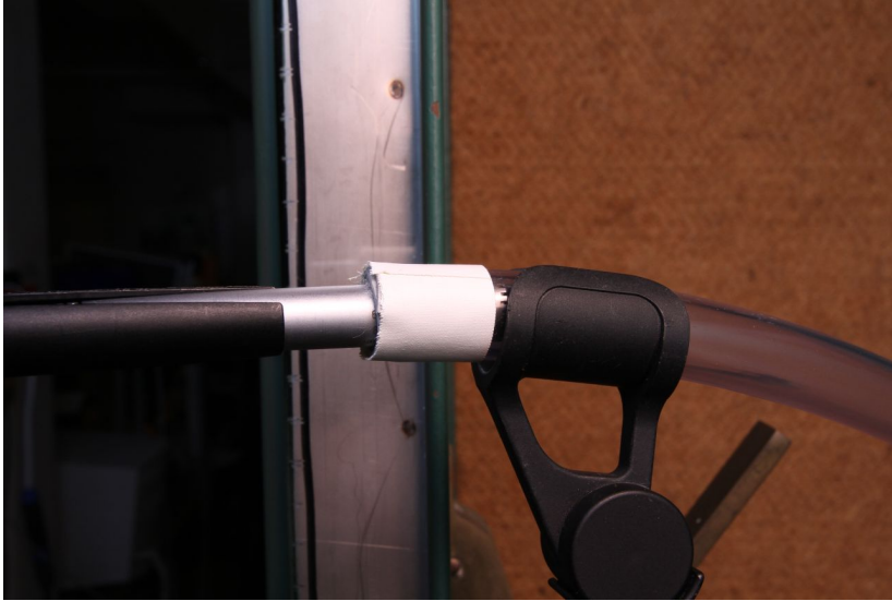
Figure 2.31. Insulated microphone end of the tube extender
