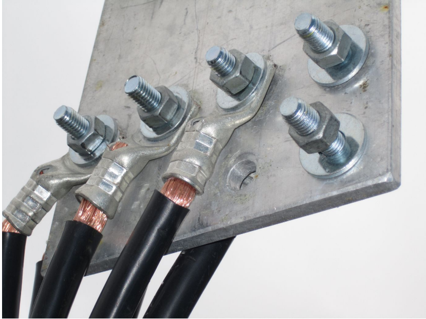
Figure 2.48. Finally loose bolts were added near the input to see if they create noise
