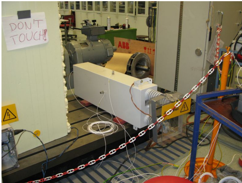
Figure 2.19. Capacitor in the standard installation position
