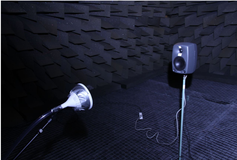
Figure 2.29. Overview of the tube extender response measurement
