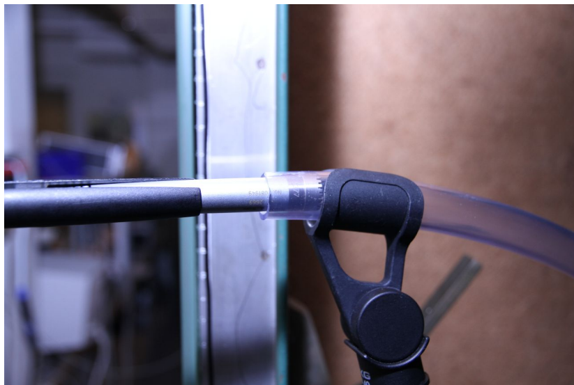
Figure 2.30. Microphone end of the tube extender
