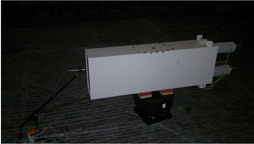
Figure 2.22. Close-up of the capacitor during the acoustic measurements
