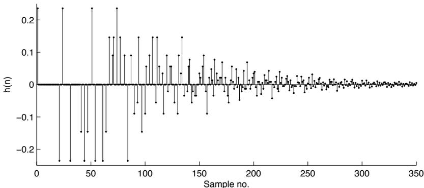
**Figure 3.3.** Impulse response of a cascade of three first-order allpass filters, with allpass coefficient  $g = \pm 0.618$  and delay-lengths of 20, 23 and 30 samples.
