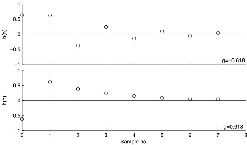
**Figure 3.1.** First 8 samples of the impulse response of a first-order allpass filter, with golden-ratio allpass coefficient  $g = \pm 0.618$ .
