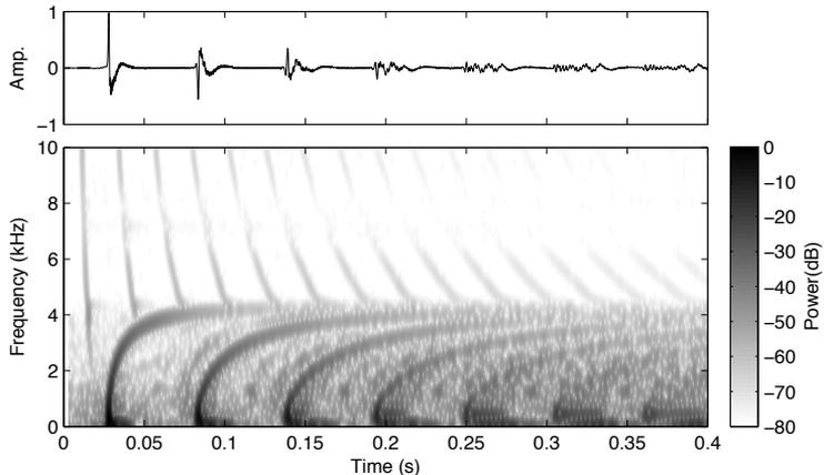
**Figure 4.2.** Impulse response of typical spring used for spring reverberation, presented in time-domain and as spectrogram.
