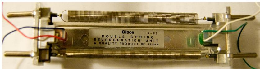
**Figure 4.1.** Typical spring reverberation unit.
