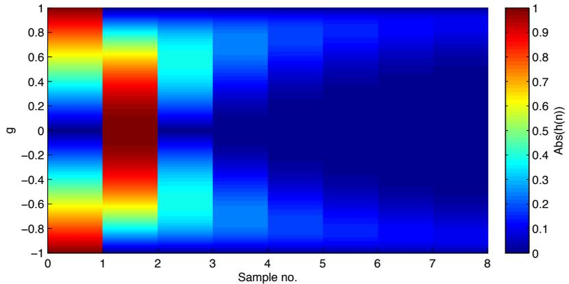
**Figure 3.2.** Diagram showing absolute value of the first 8 samples of the impulse response of a first-order allpass filter, with varying values of allpass coefficient  $g$ .
